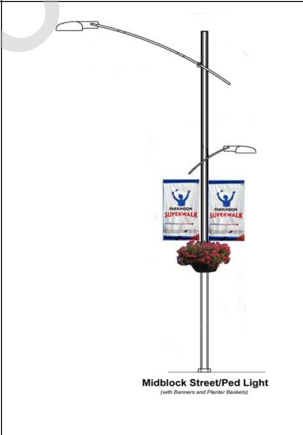
FIGURE C3-5 STREET SIGNAL/LIGHTING SYSTEM (NOT TO SCALE)
