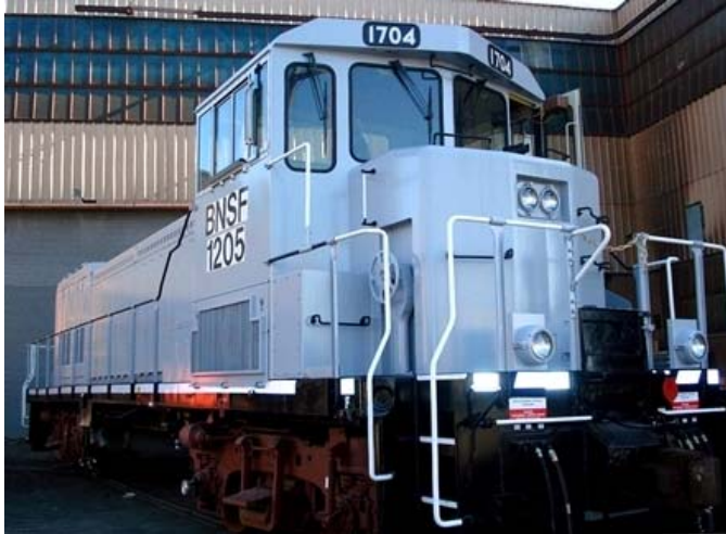
Figure 3-13 - Experimental BNSF Fuel Cell Switch Engine
