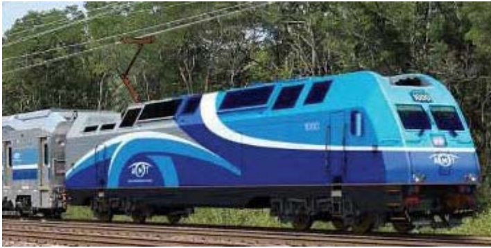
Figure 3-8 - Rendering of the Dual-Mode Locomotive ALP45DP
