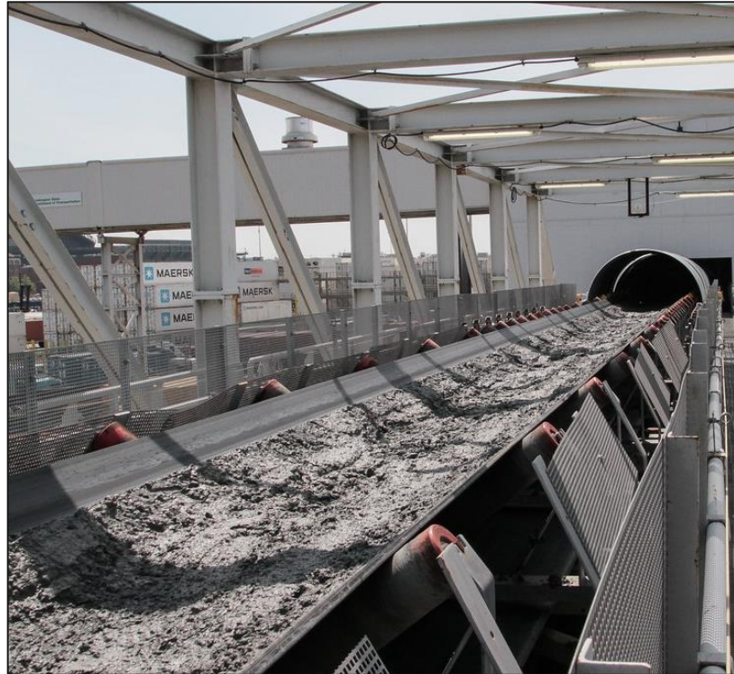
Left: An example of a muck conveyor to support tunneling. Right: The area at the east end of the site where foundational construction is occurring for the muck conveyor system.
