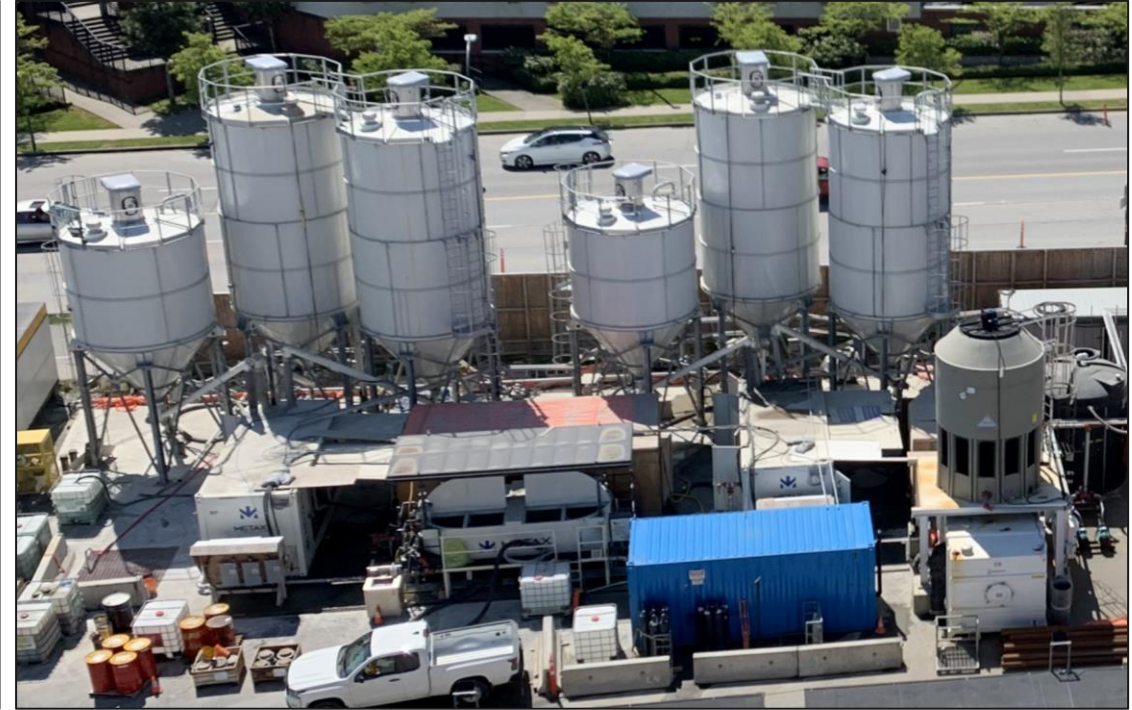
Left: Crews prepare the foundation of the plant, to the east of the portal. Right: An example of a grout plant, used in Vancouver, B.C.
