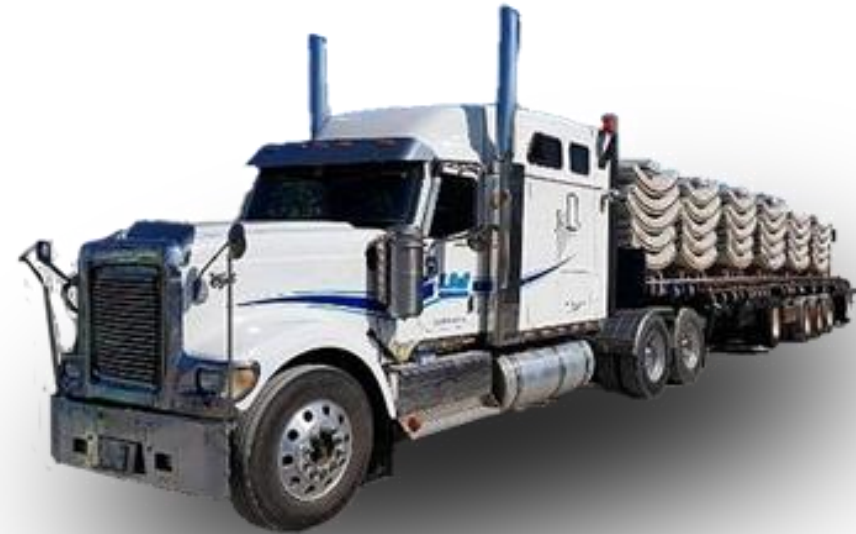
Flatbed transport with pre-cast tunnel segments
