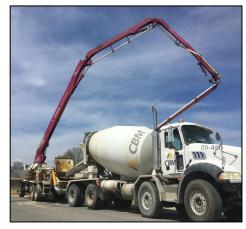
Concrete and Pump Trucks deliver and distribute concrete to hard-to-reach areas like deep foundational holes.
