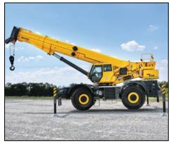
Temporarily stationed on-site during equipment assembly/disassembly, **mobile cranes** lift and move heavy materials, such as steel beam and concrete segments.
