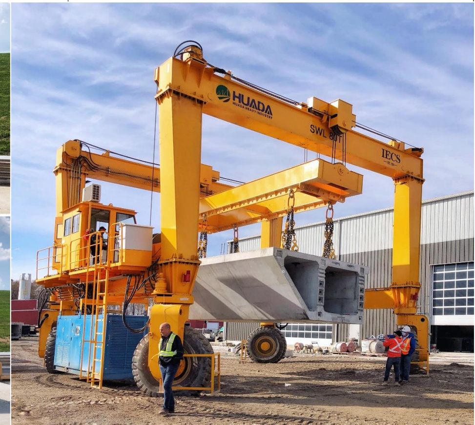
Bridge span segment at the manufacturing facility
