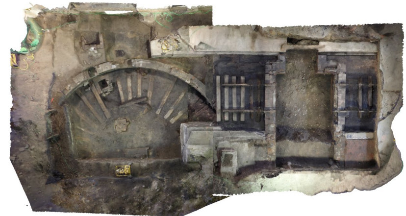
Photogrammetric model of First Parliament site remains, showing a 19 th century railway turntable and rail line dating to after the Parliament buildings during the use of the site by Consumers' Gas.
