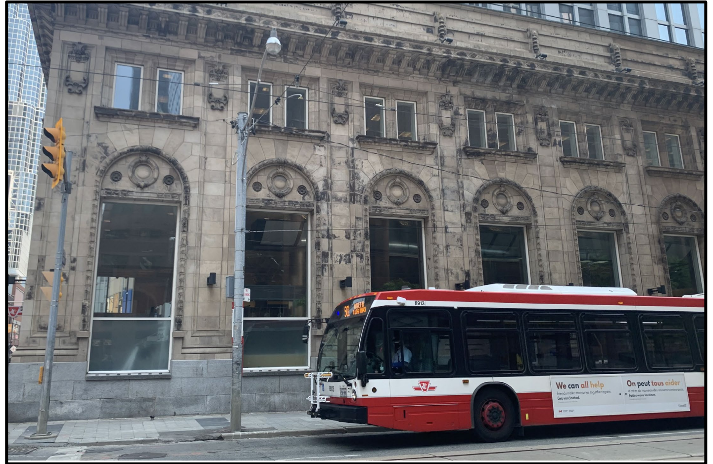
Two Queen East is a great example of a site where heritage façades have been conserved, attached to a newer, larger structure, with TTC subway entrances.
