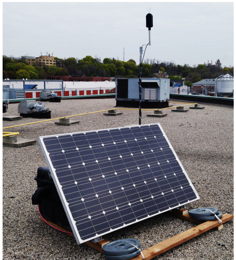
Long-term construction noise monitoring station, with solar power and remote telecommunications
