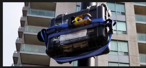
Noise logger capturing ambient noise
