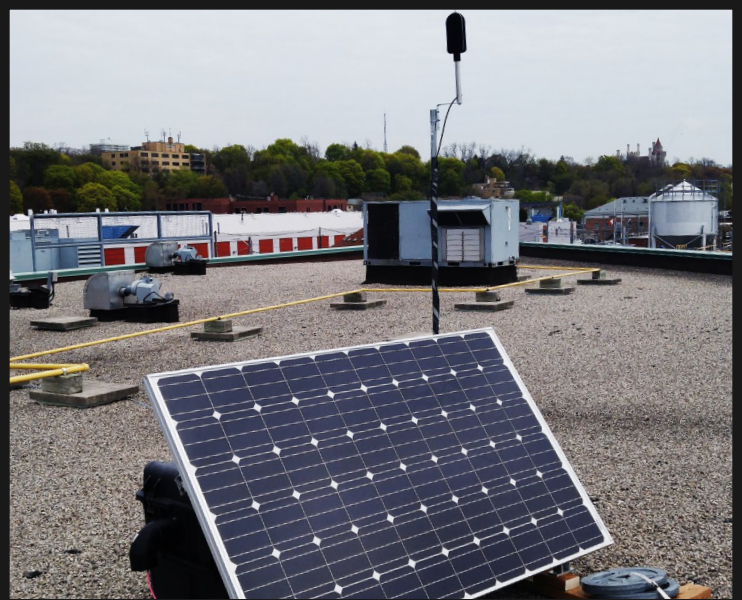
Long-term construction noise monitoring station, with solar power and remote telecommunications
