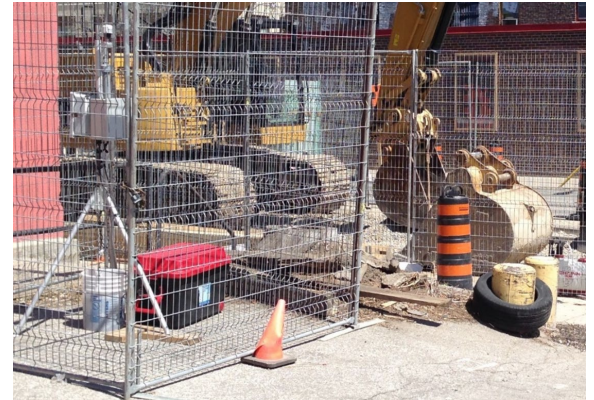
Example of construction dust monitor in a fenced enclosure (left side of photo)
