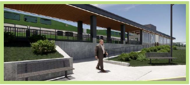
As part of the accessibility upgrades at Eglinton GO Station, barrier-free accessible ramps and walkways with heat-traced ramps for snow melt will be added. Artist's rendering, final designs are subject to change. (Metrolinx image).
