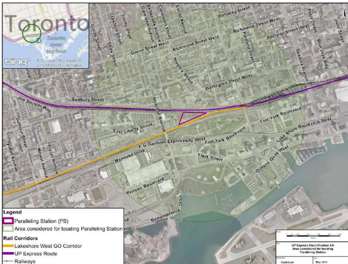
Figure 2-2 Alternative Sites for Paralleling Station in Bathurst Street and UP Express route/corridor
