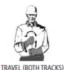
Rotate fists around each other in front of body; direction of rotation away from body indicates travel forward; rotation towards body indicates travel backward. (For crawler cranes only)
