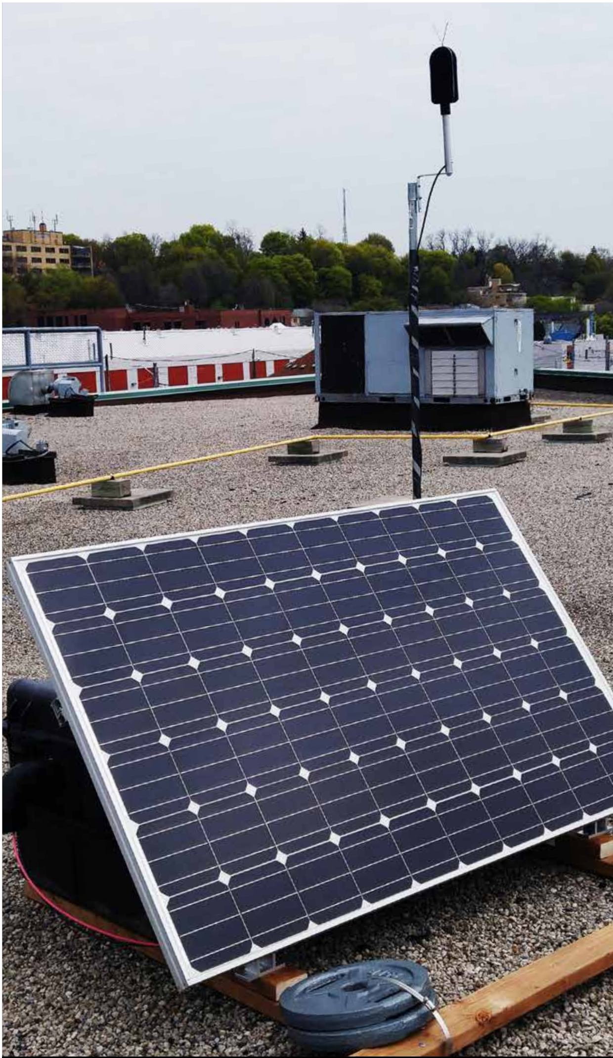
Long-term construction noise monitoring station, with solar power and remote telecommunications
