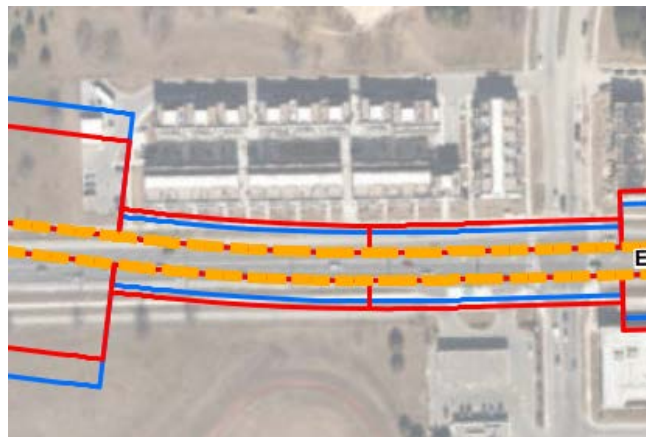
Figure 8-9: Alignment Centreline showing Ground-borne Vibration (blue) and Noise (red) Contours near 99+800 and 99+700 with Mitigation
