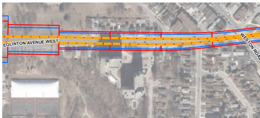
Figure 8-6: Alignment Centreline showing Ground-borne Vibration and Noise Contours near 105+500 to 105+200 with Mitigation
