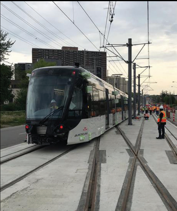
Photo: Testing and Commissioning team members carefully observe the LRV making its journey along the burn-in track.
