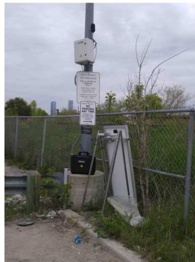
Example of a construction noise monitor. Source: AECOM, 2017.
