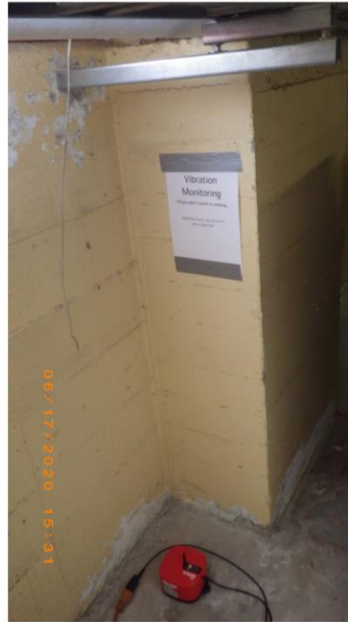
Example of a construction vibration monitor. Source: AECOM, 2020.
