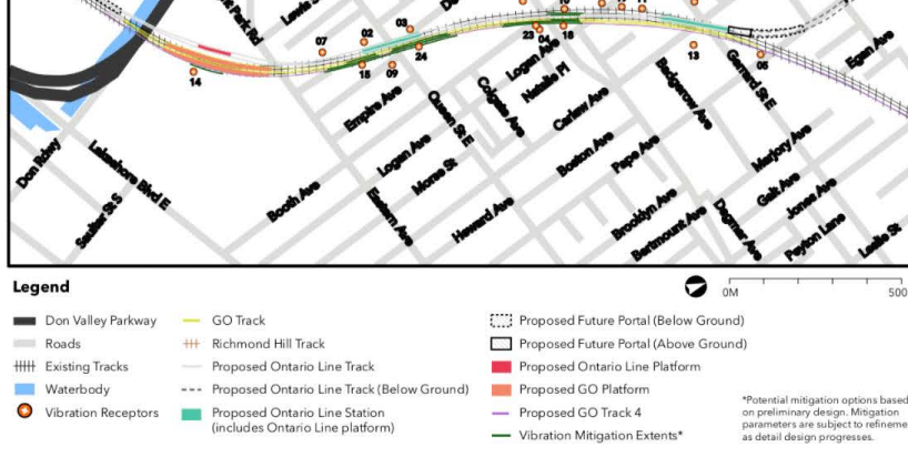
Map showing the proposed Ontario Line and GO tracks through the Lakeshore East corridor, highlighting vibration mitigation extents.
