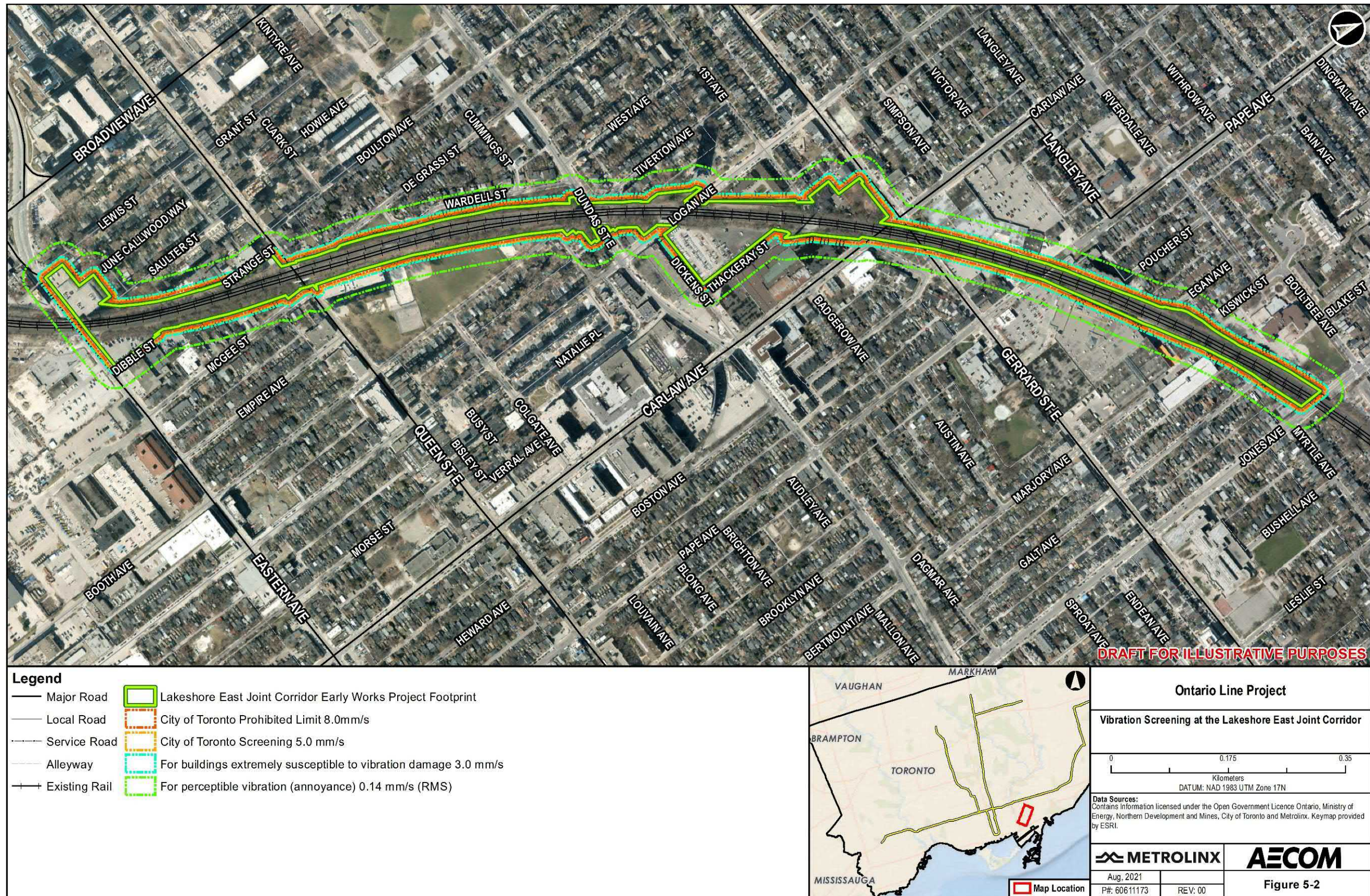
Figure 5-2: Vibration Screening for the Lakeshore East Joint Corridor Early Works Project Footprint
