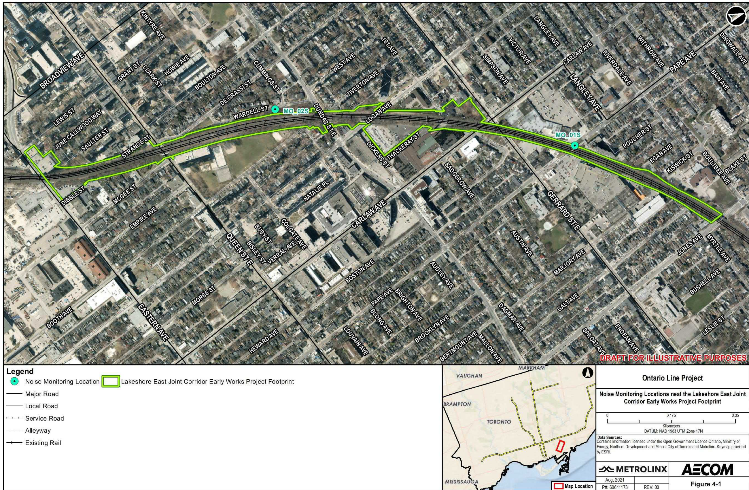
Figure 4-1: Noise Monitoring Locations near the Lakeshore East Joint Corridor Early Works Project Footprint
