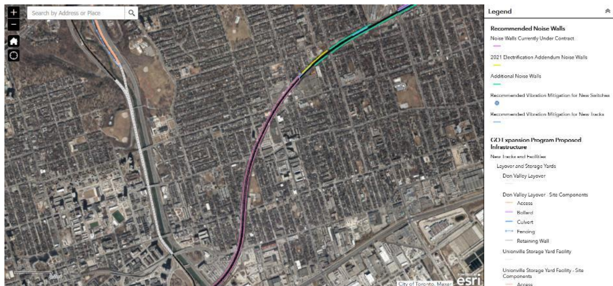
Figure 2-3: Recommended noise walls and vibration mitigation for GO service expansion between Greenwood and the Don Valley (Source: GO Expansion Program Public Consultation Meeting 3 rd Round November-December 2020, accessed 2021-06-19 )
