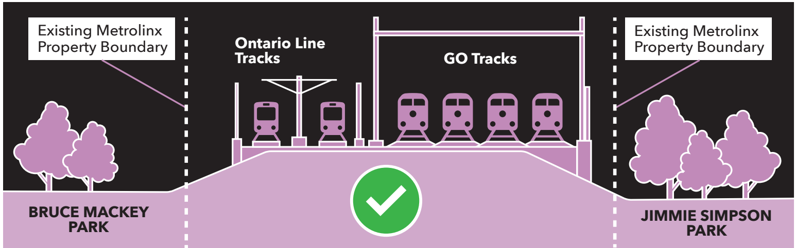
TRUE-TO-PLAN METROLINX CROSS SECTION WITH BOTH ONTARIO LINE AND GO SERVICES WITHIN EXISTING PROPERTY BOUNDARIES (NORTH OF REC CENTRE)
