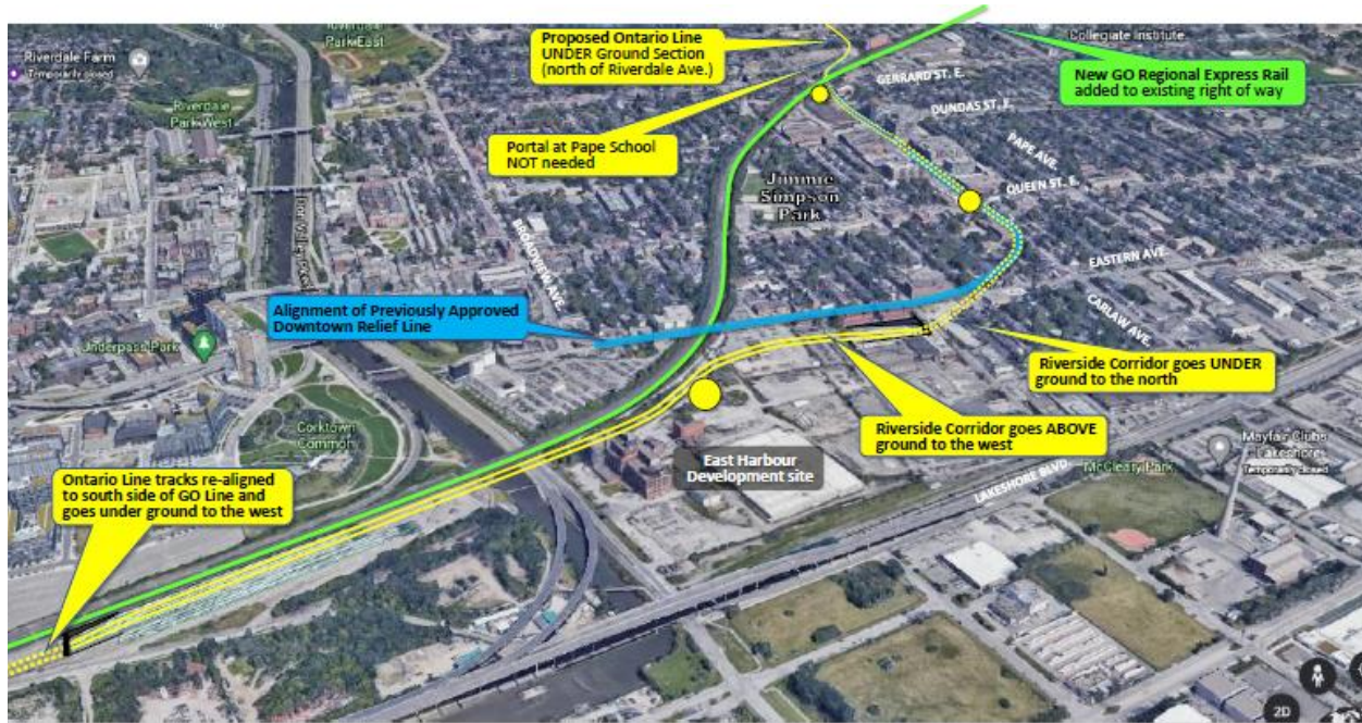
Figure 1-6: An alternative underground alignment for the Ontario Line as proposed by the Riverside and Leslieville communities
