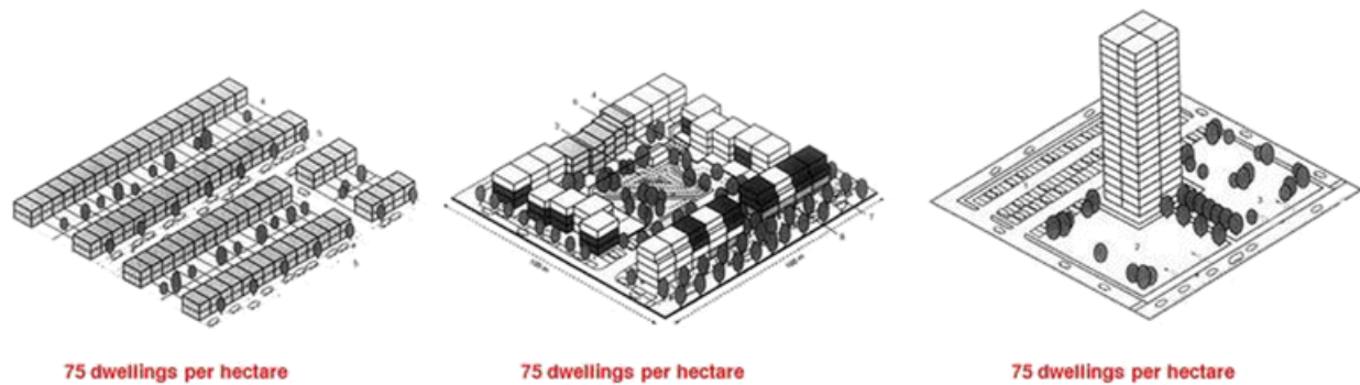
Figure 2-13: Achieving housing density per hectare using low-rise, mid-rise and high-rise building forms (Source: Lehmann 2016)
