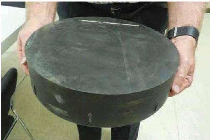
These rubber discs are used along the western portion of Line 1 to cushion the concrete slabs that supports the subway tracks from the tunnel walls, further absorbing vibrations. (Image courtesy of the Toronto Transit Commission)
