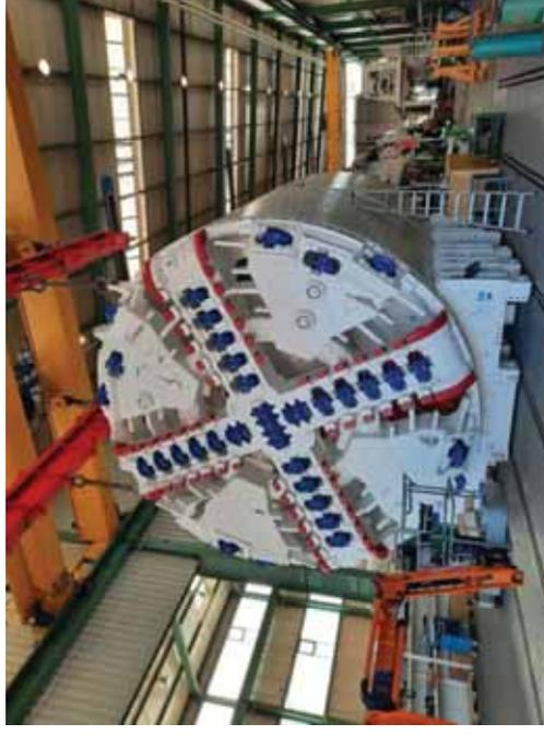
One of the Eglinton Crosstown West Extension TBMs during factory testing in Germany (West End Connectors photo)
