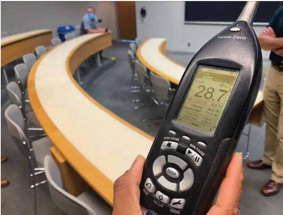
A baseline sound level reading is captured in the lecture hall by an acoustic monitoring device. (Metrolinx photo)
