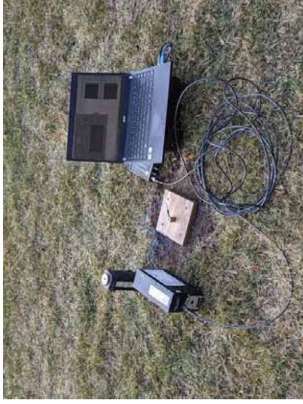
Example of construction vibration monitoring station set up outdoors for short-term measurements. Long-term monitoring station would be similar and enclosed in a weather-proof box with solar power connection.
