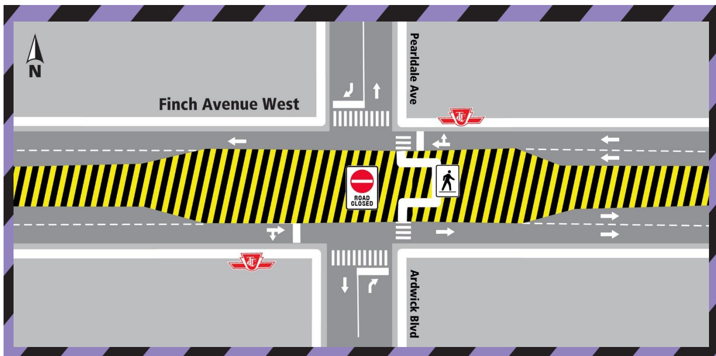
Road Configuration for Stage 1 and 2
