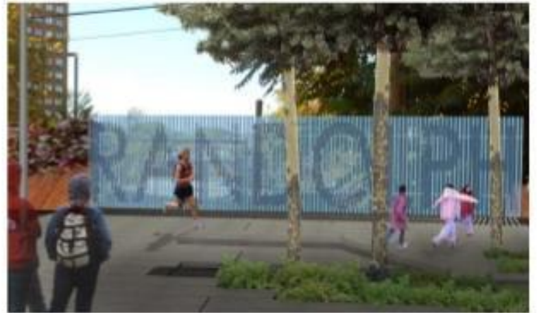
Street ending terminus signage to be part of artwork strategy. Signage to be semi-transparent adhesive overlayed on acrylic noisewall panel.
