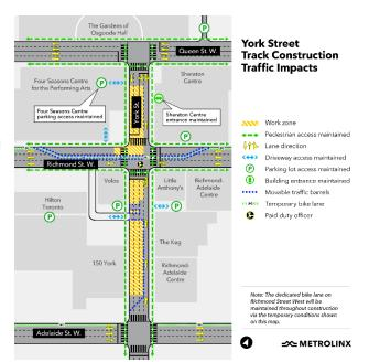
excavation, pouring of a track slab foundation, and conducting work on the traffic signals to support the installation of new streetcar tracks.
