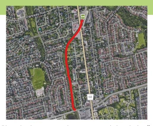
Metrolinx will be undertaking routine track maintenance work along the Stouffville rail corridor near Markham GO Station and 16<sup>th</sup> Avenue. As part of this work, we will be undercutting the tracks to remove and replace old ballasts (the material that supports track stability), to ensure proper drainage and a strong foundation. This work will be conducted by our corridor maintenance team, and it is necessary to keep our infrastructure in good shape.
