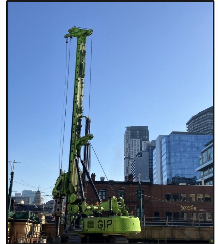
Example of a drilling machine used in piling construction
