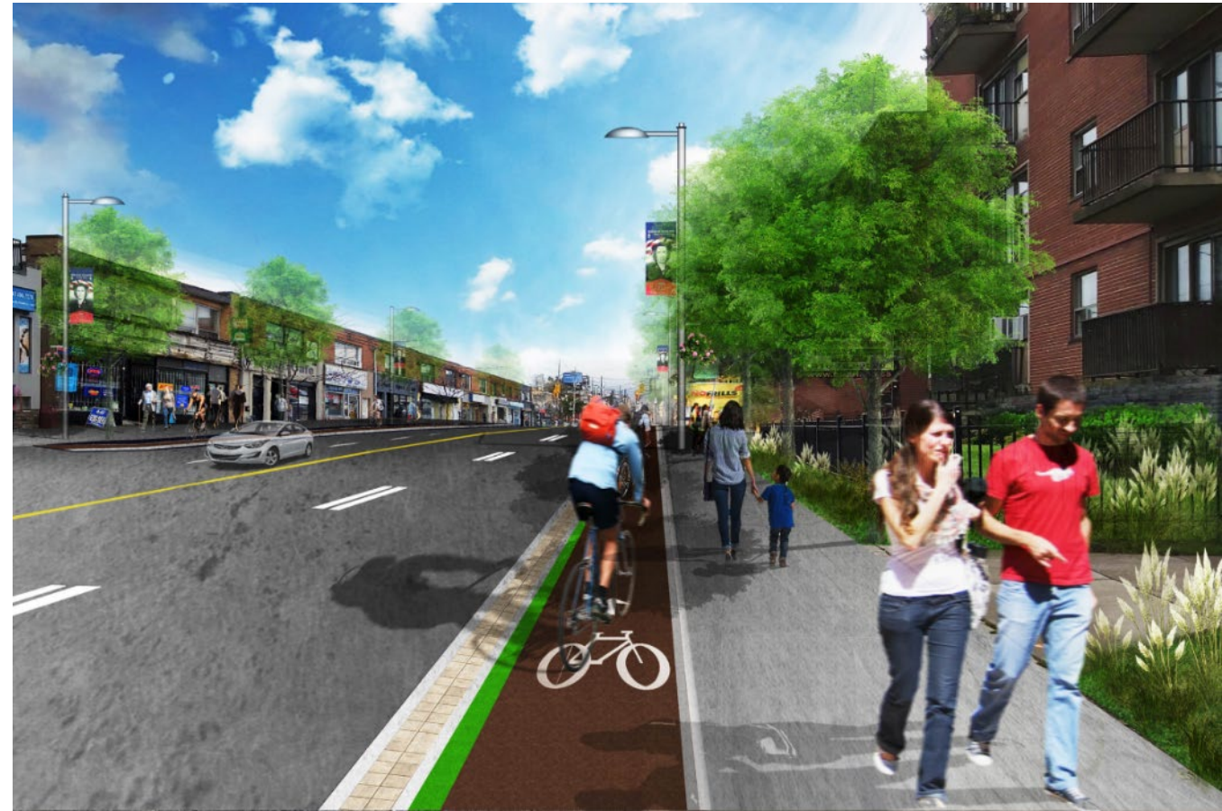
Sample rendering of a raised cycle track and sidewalk.
