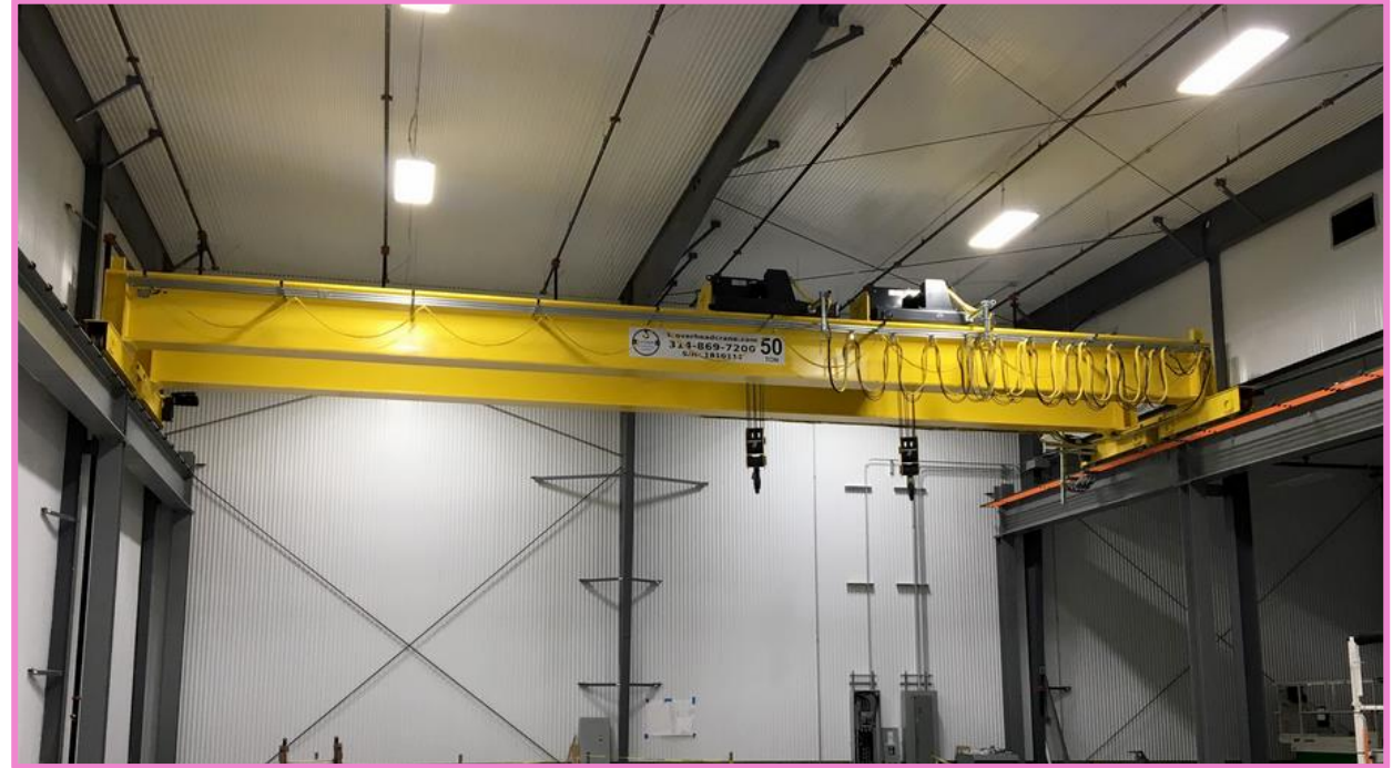
Example of an overhead crane; a mobile crane to help hoisting operations within the long-term acoustic shelter.
