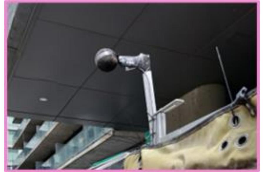
*Example of a type of noise monitoring device.*
