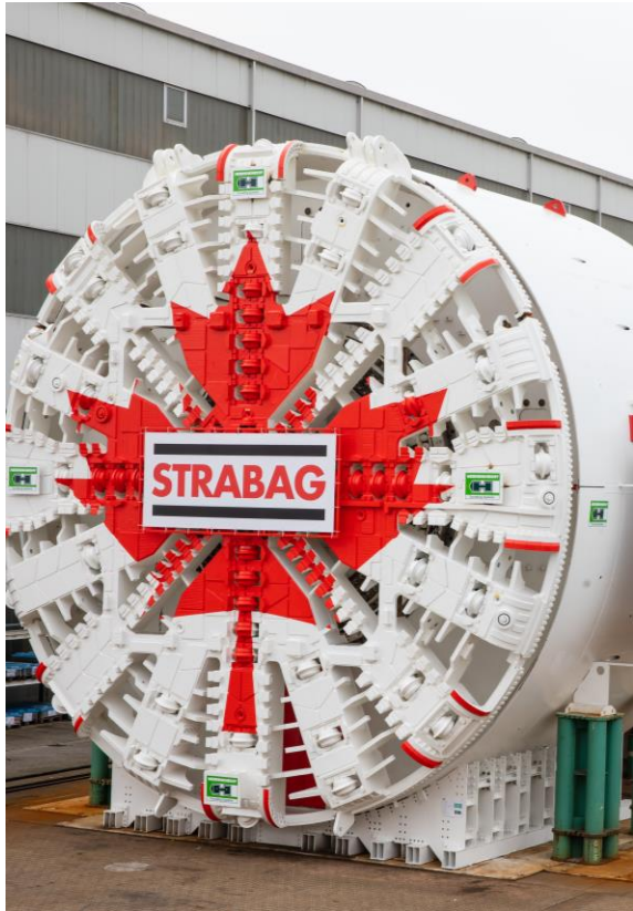
MEET DIGGY SCARDUST , A TUNNEL BORING MACHINE USED TO CREATE THE TUNNEL FOR THE FUTURE SUBWAY EXTENSION IN SCARBOROUGH.
