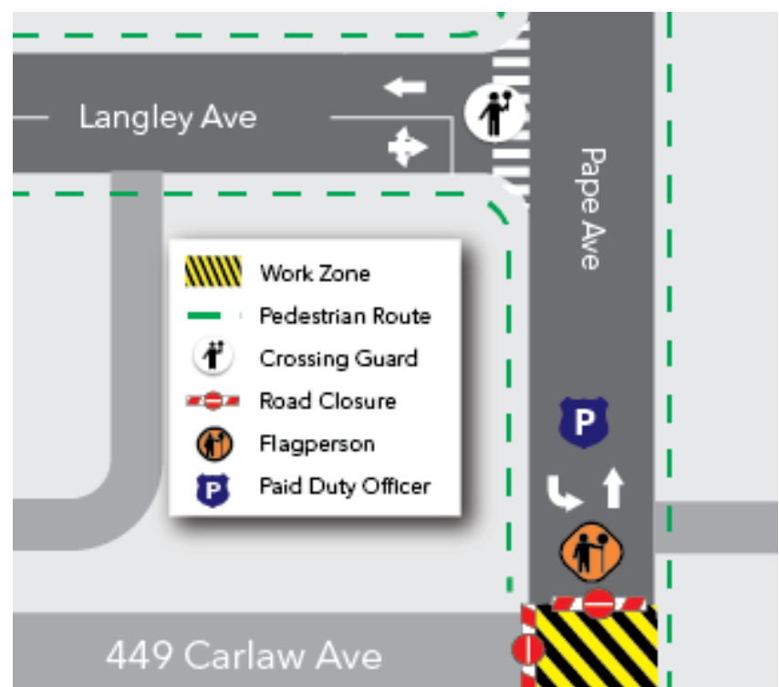
Road occupancy at foot of Pape Avenue and plaza access closure
