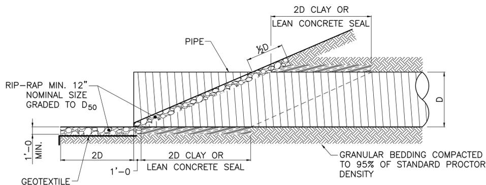
INORGANIC CLAY OR LEAN CONCRETE SEAL TO BE PLACED AT BOTH ENDS OF CULVERTS FOR A LENGTH OF TWICE THE DIAMETER (2D). THE CLAY OR LEAN CONCRETE SEAL SHALL EXTEND FROM THE BOTTOM OF THE EXCAVATION TO 12" ABOVE THE CROWN OF THE PIPE AND FOR THE FULL WIDTH OF THE EXCAVATION.
