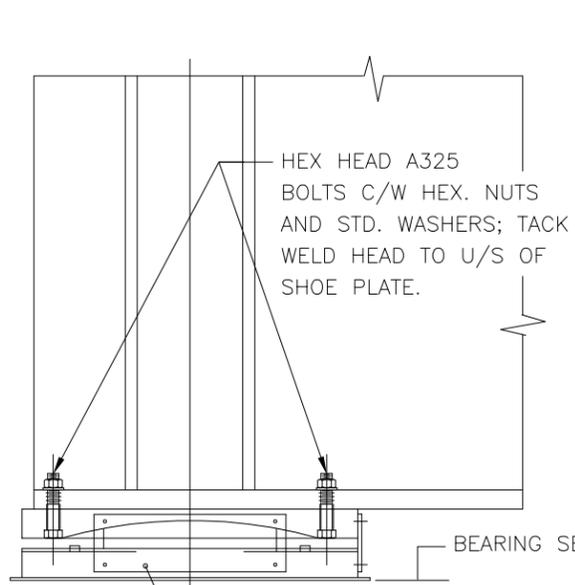
BEARINGS SHALL BE SHIPPED ASSEMBLED WITH PLATES 8 AND M16 MACHINE BOLTS. PLATES SHALL BE REMOVED AFTER ANCHOR BOLTS HAVE BEEN INSTALLED.(3 PLATES PER BEARING)
