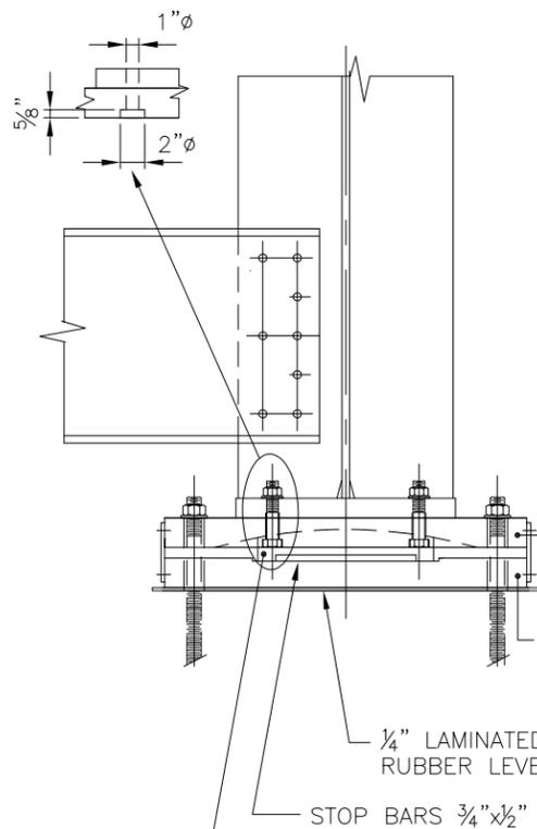
BRONZE PLATE SELF LUBRICATING WITH "X" mm RADIUS SPHERICAL TOP TOLERANCE: -0.01", +0.00" BEARINGS "F" - LUBRICATE TOP ONLY BEARINGS "E<sub>x</sub>", "E<sub>y</sub>" & "E<sub>xy</sub>" - LUBRICATE TOP & BOTTOM.
