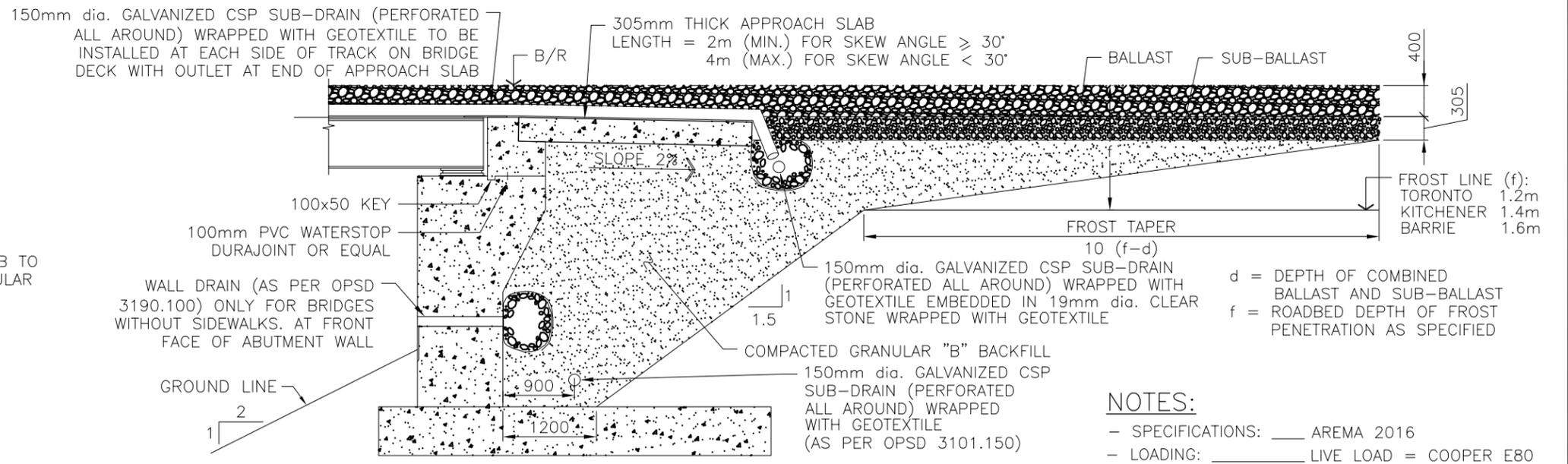
MIN. GRANULAR BACKFILL REQUIREMENTS
