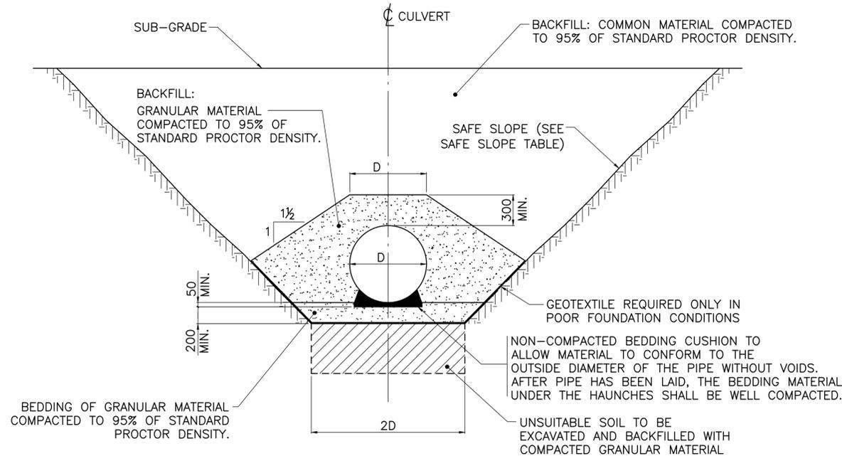
GRANULAR MATERIAL FOR BEDDING AND BACKFILLING TO BE APPROVED BY THE ENGINEER. IN GENERAL, PIT-RUN SAND AND GRAVEL, REASONABLY WELL GRADED FROM MAXIMUM SIZE 100mm TO NOT MORE THAN 8% FINER THAN SIEVE No. 200.
