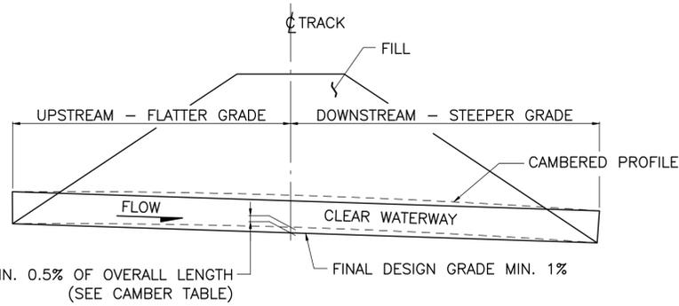
**MINIMUM GRADE AND CAMBERING REQUIREMENTS FOR CULVERT INSTALLATION**
