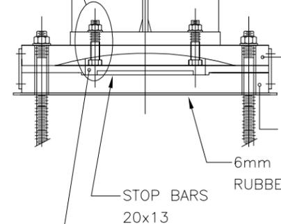
BRONZE PLATE SELF LUBRICATING WITH "X" mm RADIUS SPHERICAL TOP TOLERANCE: -0.25mm, +0.00mm. BEARINGS "F" - LUBRICATE TOP ONLY BEARINGS "E<sub>x</sub>", "E<sub>y</sub>" & "E<sub>xy</sub>" - LUBRICATE TOP & BOTTOM.
