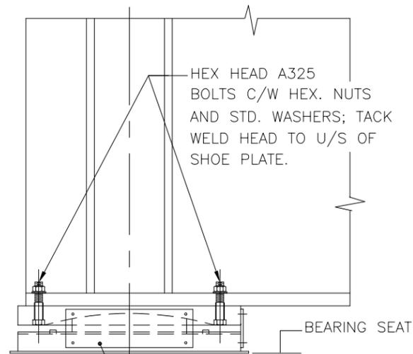
BEARINGS SHALL BE SHIPPED ASSEMBLED WITH  $\frac{5}{16}$ " PLATES AND  $\frac{5}{8}$ " $\phi$  MACHINE BOLTS. PLATES SHALL BE REMOVED AFTER ANCHOR BOLTS HAVE BEEN INSTALLED.(3 PLATES PER BEARING)
