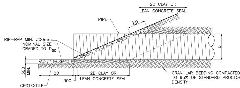
INORGANIC CLAY OR LEAN CONCRETE SEAL TO BE PLACED AT BOTH ENDS OF CULVERTS FOR A LENGTH OF TWICE THE DIAMETER (2D). THE CLAY OR LEAN CONCRETE SEAL SHALL EXTEND FROM THE BOTTOM OF THE EXCAVATION TO 300mm ABOVE THE CROWN OF THE PIPE AND FOR THE FULL WIDTH OF THE EXCAVATION.
