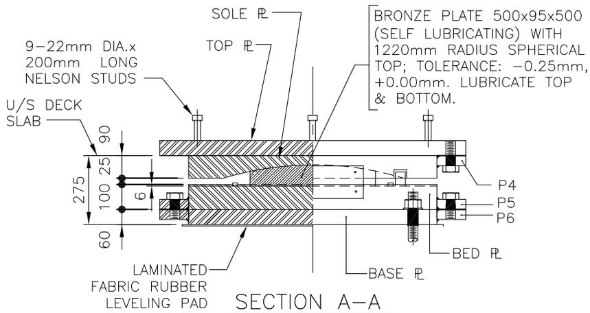
BEARINGS SHALL BE SHIPPED ASSEMBLED
