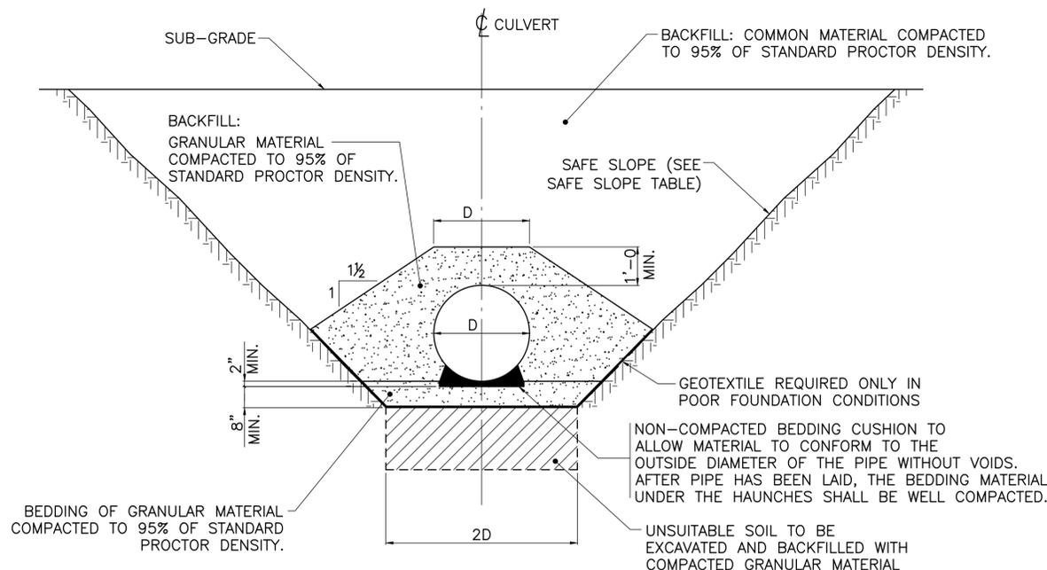
GRANULAR MATERIAL FOR BEDDING AND BACKFILLING TO BE APPROVED BY THE ENGINEER. IN GENERAL, PIT-RUN SAND AND GRAVEL, REASONABLY WELL GRADED FROM MAXIMUM SIZE 4" TO NOT MORE THAN 8% FINER THAN SIEVE No. 200.
