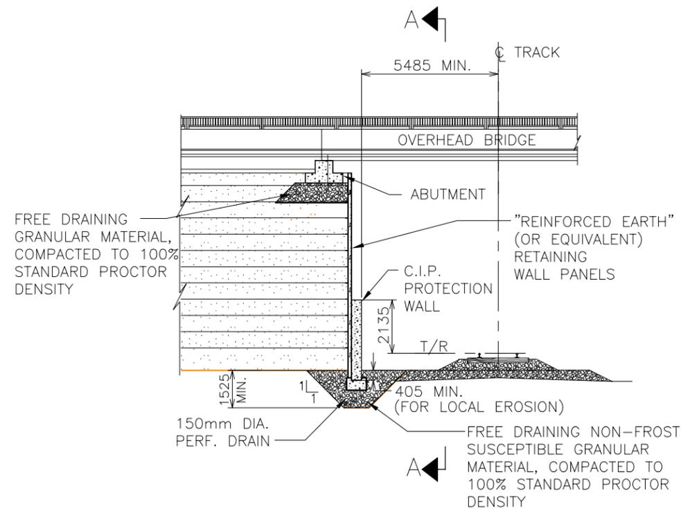
TYPICAL SECTION FOR ABUTMENTS ON GRANULAR BASE
