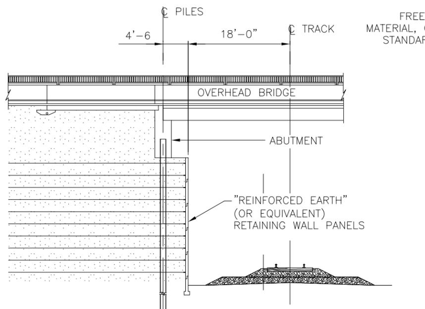
TYPICAL SECTION FOR ABUTMENTS ON PILES
