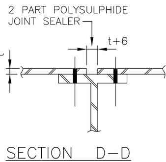
NOTE: USE E 7018 ELECTRODE OR EQUIVALENT FOR WELDS SHOWN.
