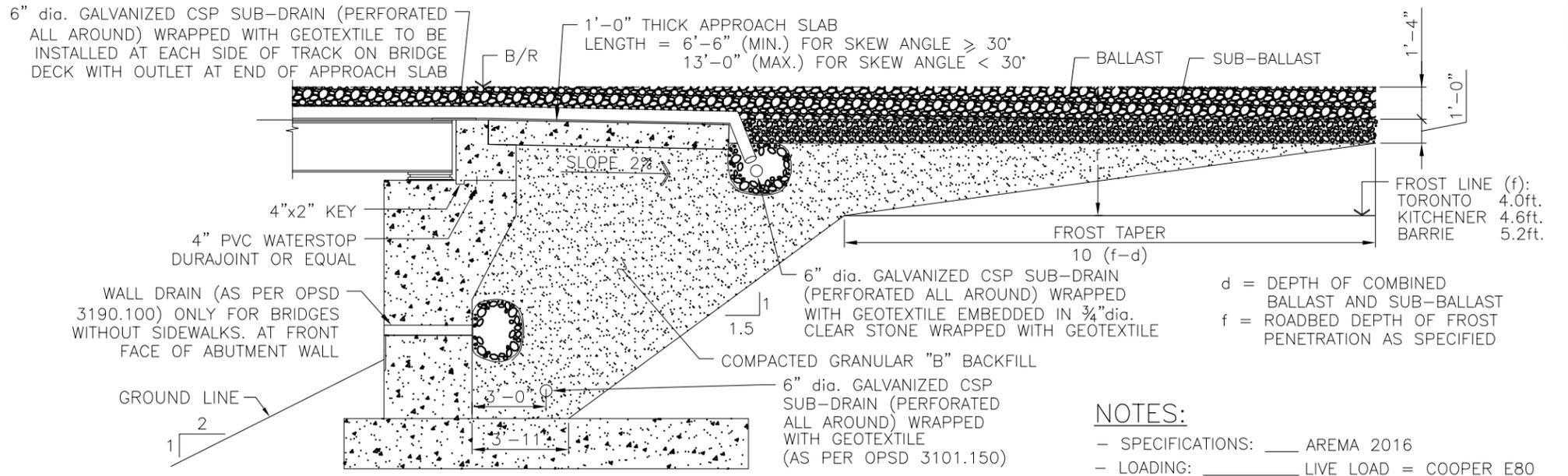
MIN. GRANULAR BACKFILL REQUIREMENTS
