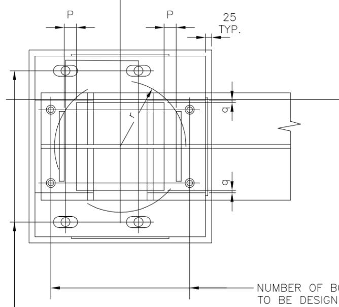
HOLES IN SHOE & BED PL & LEVELING PAD FOR M30Ø OR M36Ø ANCHOR BOLTS AS PER CN STD. S3A. FOR SIZES OF HOLES SEE DWG. NO. S-16.
