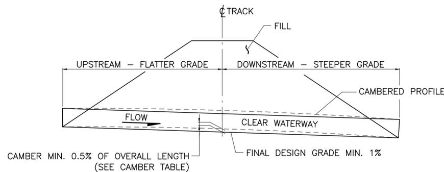
**MINIMUM GRADE AND CAMBERING REQUIREMENTS FOR CULVERT INSTALLATION**
