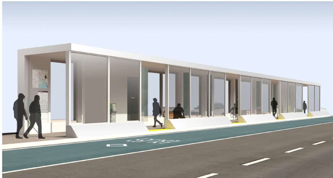
Figure 5-21: BRT pass-through shelter
