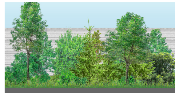
Figure 12: Vegetative screening is a key means of mitigating the negative visual impacts of noise barriers in sensitive locations such as parks and residential neighbourhoods
