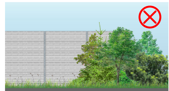
Figure 19: Noise barrier end treatment with vegetation marking termination of the structure
