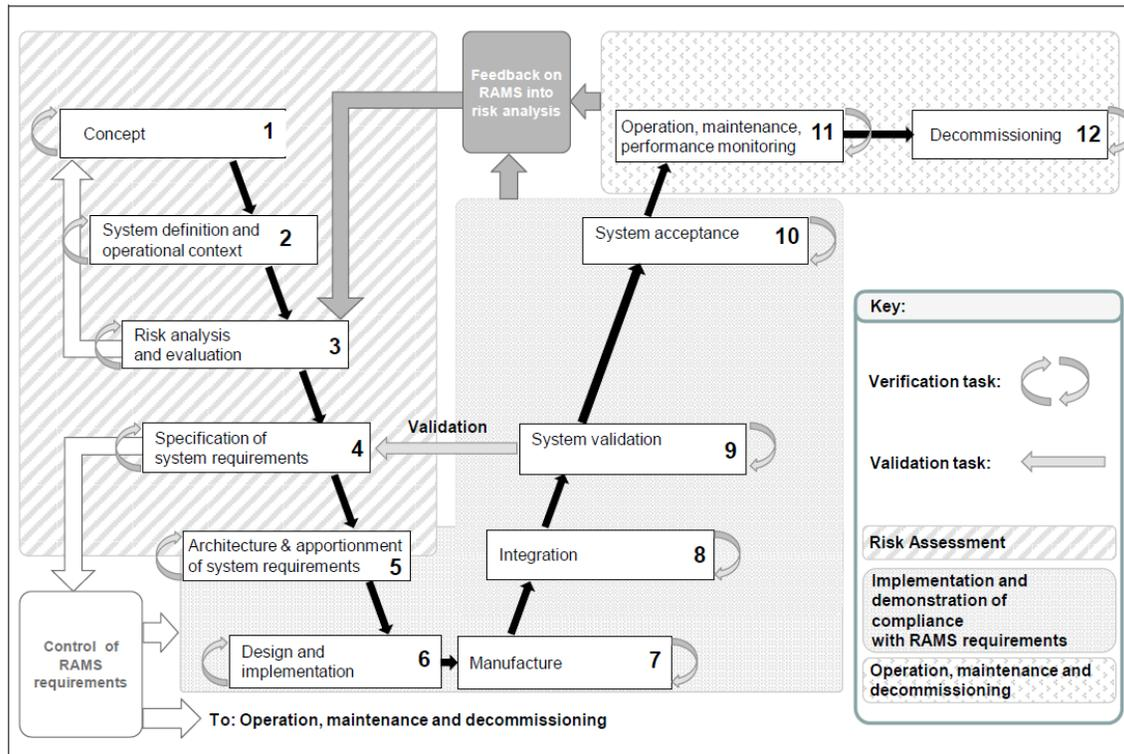
Figure 1 The interrelation of RAMS management process and system life cycle - the V-Cycle representation [Source: BS EN 50126-1:2017]<sup>1</sup>
