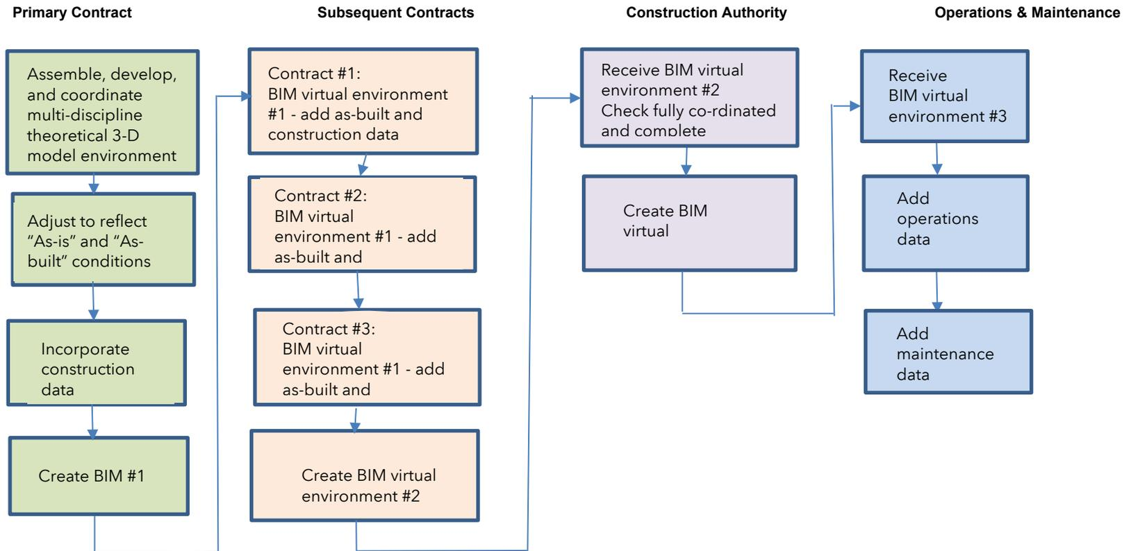
**Figure 1: BIM Data Collection Process**
