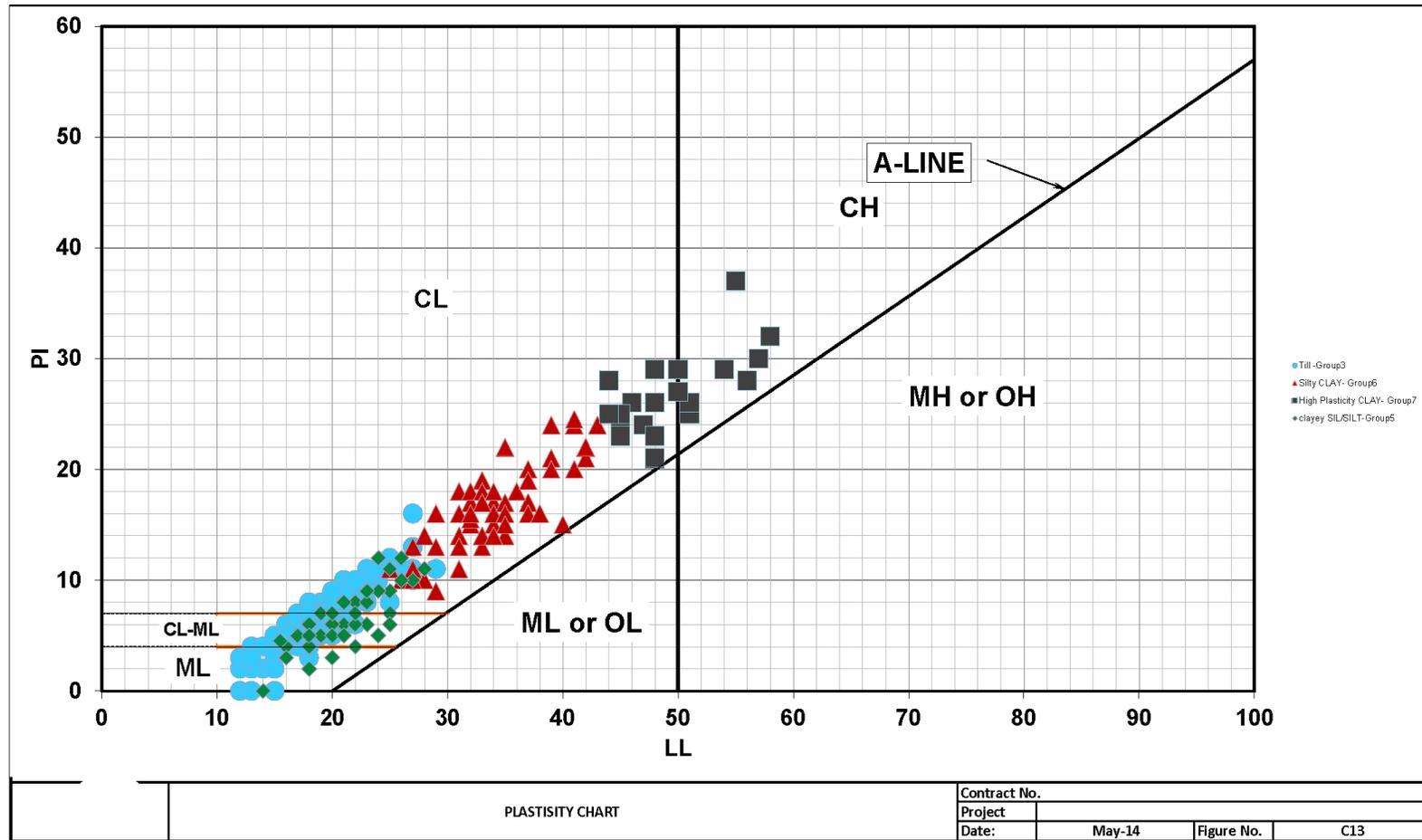
Figure 25 (C13) Atterberg Limit Envelopes for Plastic Soils
