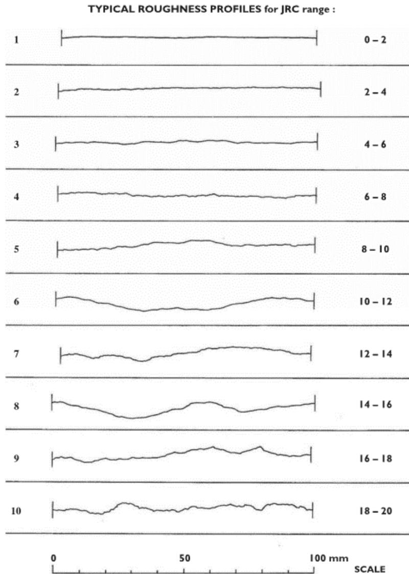
**Figure 29 Typical Roughness Profiles for JRC (Bandis et al, 1983)**
