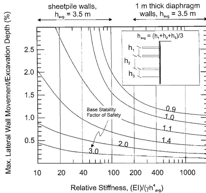
**Figure 6 Relationship between Maximum Lateral Movement and Excavation Base Stability Factor of Safety (from CFEM)**
