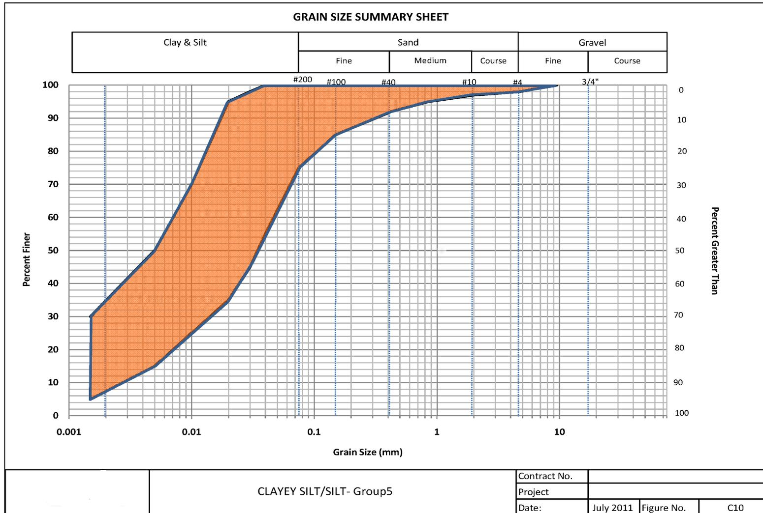
**Figure 22 (C10) Grain Size Summary Clayey Silt/Silt (Group 5)**
