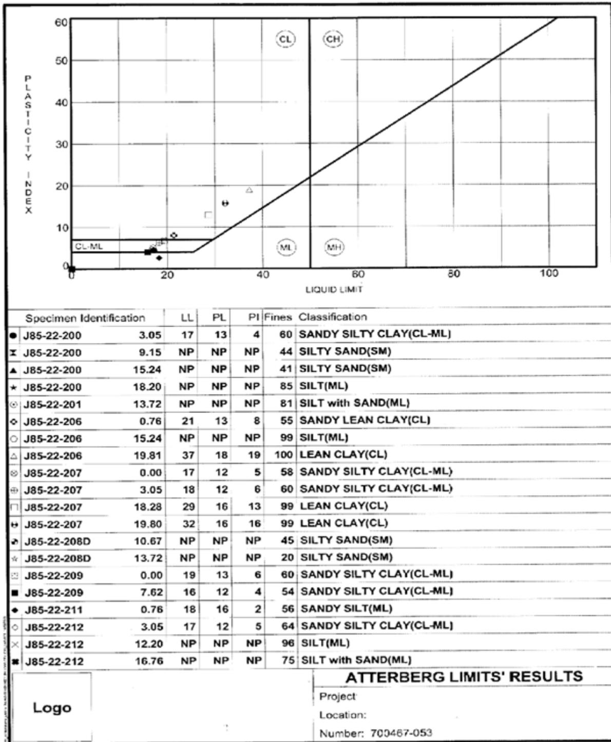
Figure 12 Example Atterberg Limits Test Results
