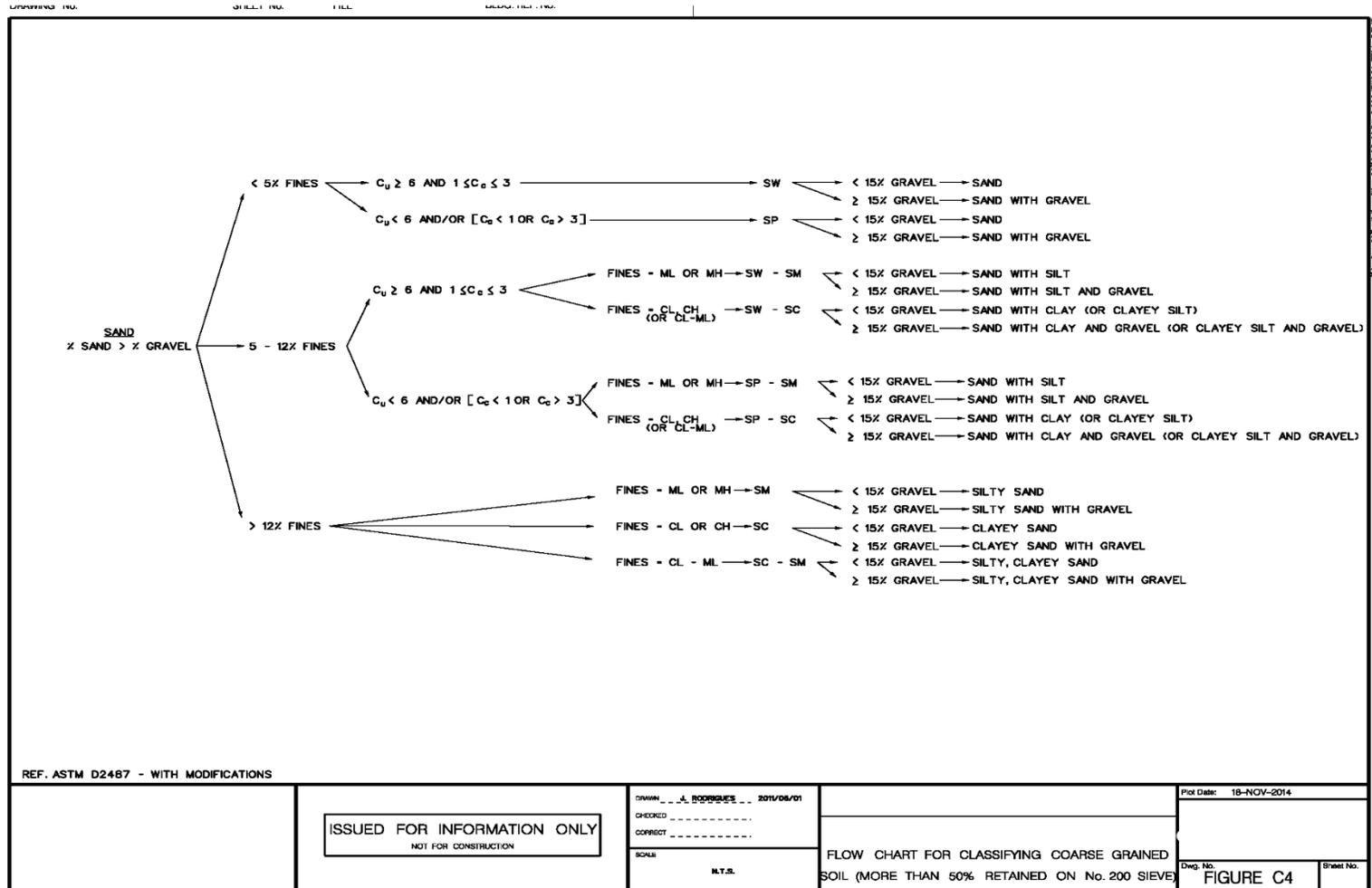
**Figure 16 (C4) Flow Chart for Classifying Coarse Grained Soils (More than 50% Retained on No. 200 Sieve)**
