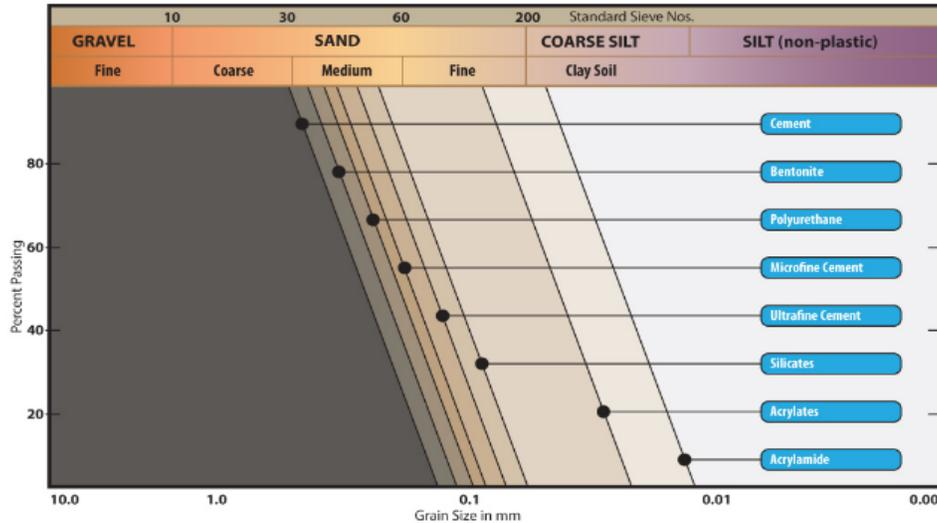
**Figure 32 Applicability of Grout Types for Permeation Grouting in Various Ground Conditions (by Avanti International)**
