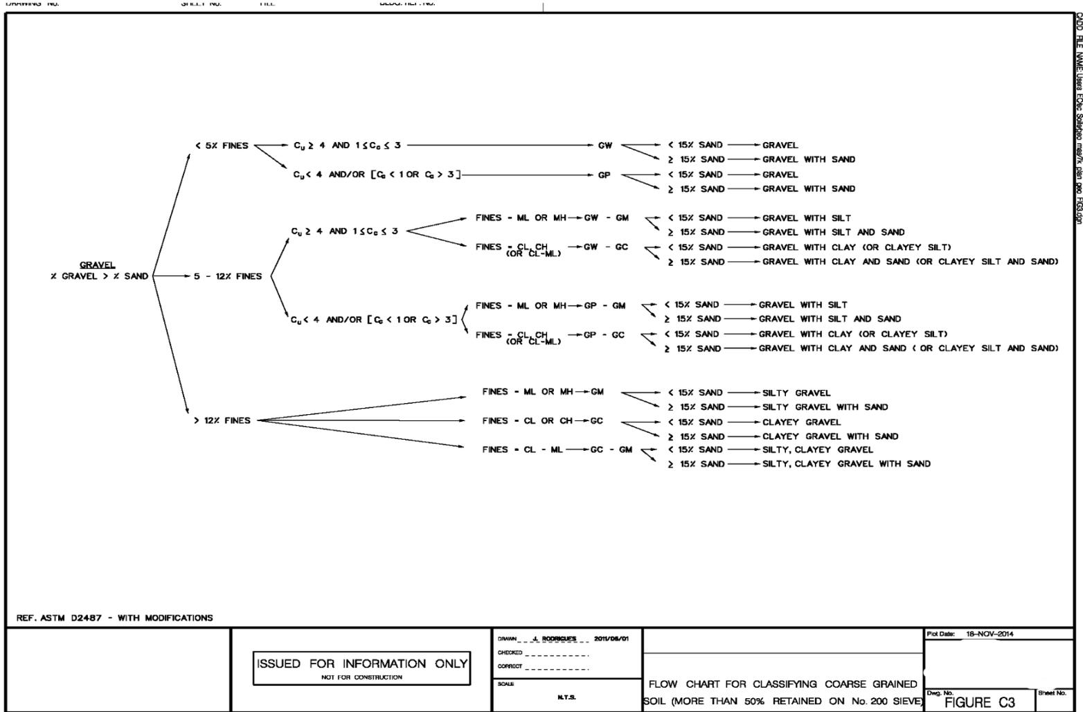
**Figure 15 (C3) Flow Chart for Classifying Coarse Grained Soils (More than 50% Retained on No. 200 Sieve)**
