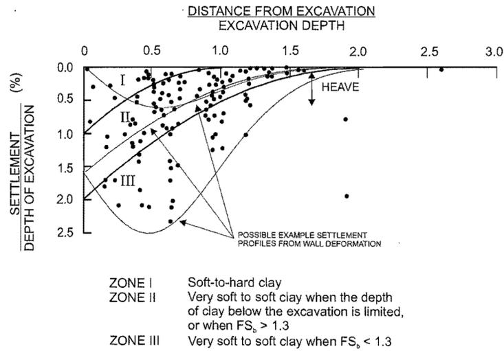
**Figure 4 Settlements Adjacent to Excavations in Soft to Medium Stiff Clay (from CFEM)**
