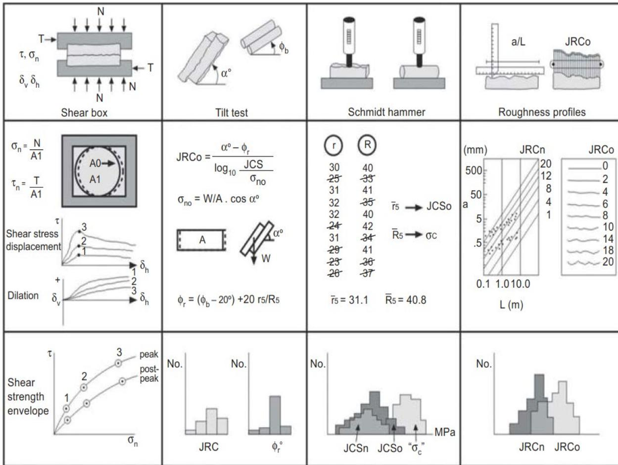
**Figure 28 Shear Box and Testing of Rock Joints**
