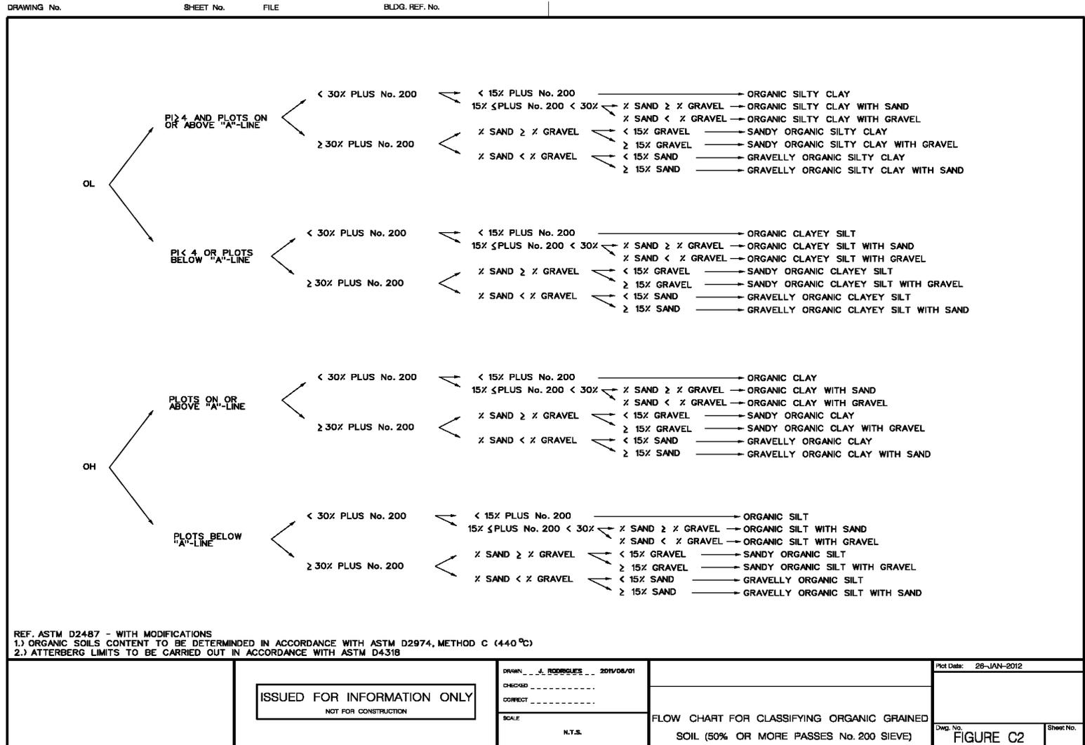
Figure 14 (C2) Flow Chart for Classifying Organic Grained Soil (50% or More Passes No. 200 Sieve)
