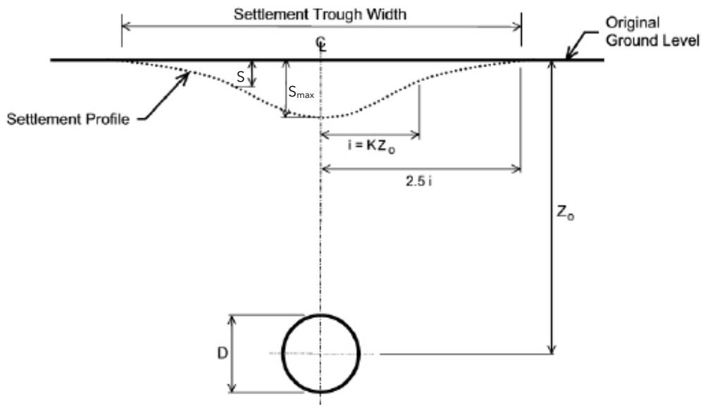
**Figure 31 Typical Settlement Profile for a Soft Ground Tunnel (from Singapore LTA)**
