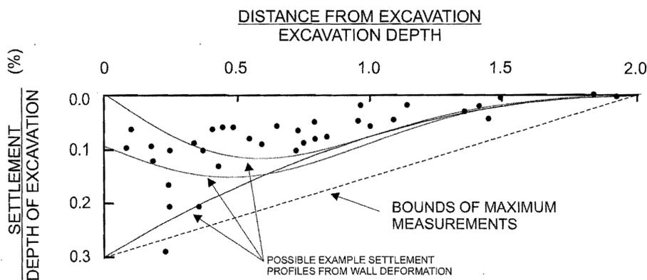
**Figure 3 Settlements Adjacent to Excavations in Sand (from CFEM)**
