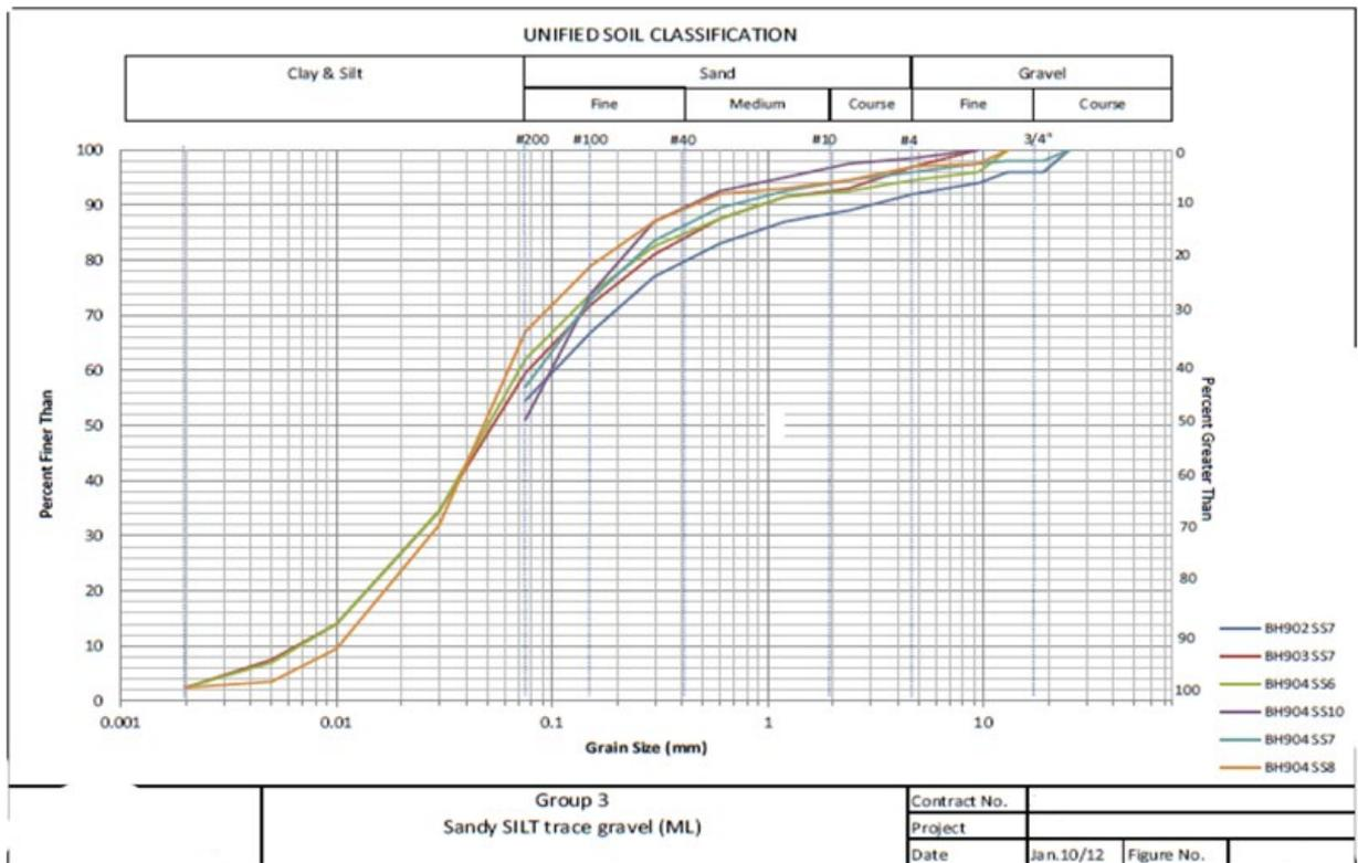
Figure 10 Example Grain Size Distribution
