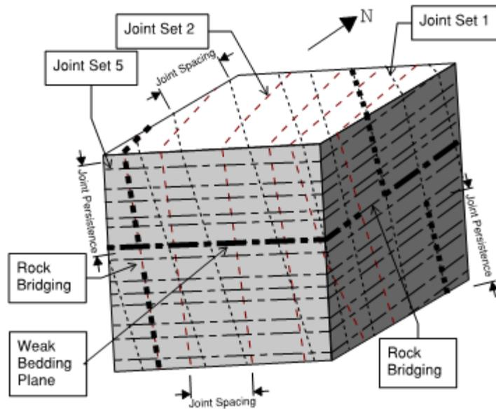
**Figure 26 Joint Spacing, Joint Persistence and Rock Bridging. (Joint sets orientations are for illustration and do not represent joint sets orientations in GBF. Diagram by Hatch)**
