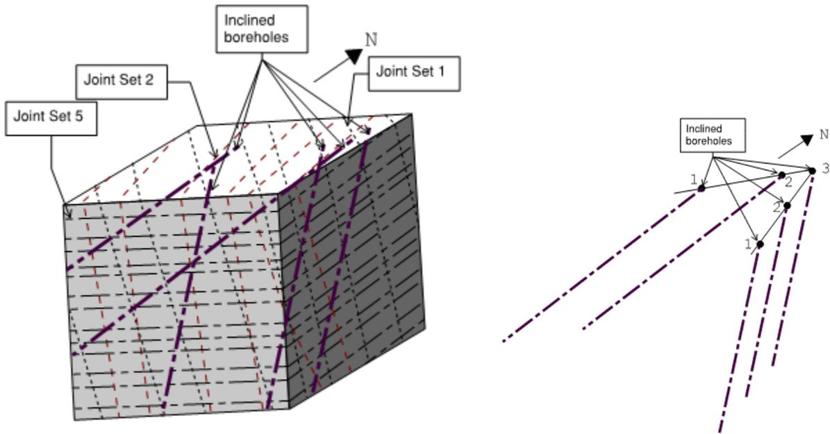
**Figure 27 Sample Bedrock Block Diagram - A Cluster of Testing Boreholes**
