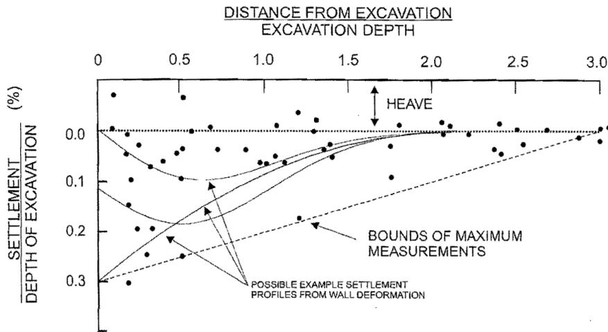
**Figure 5 Settlements Adjacent to Excavations in Stiff Clay (from CFEM)**
