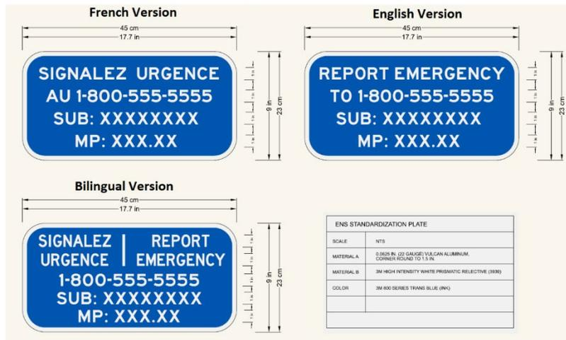
11.4.14 These signs provide crossing users with the information needed to report or notify Metrolinx about emergencies or malfunctioning warning systems or traffic control devices.
