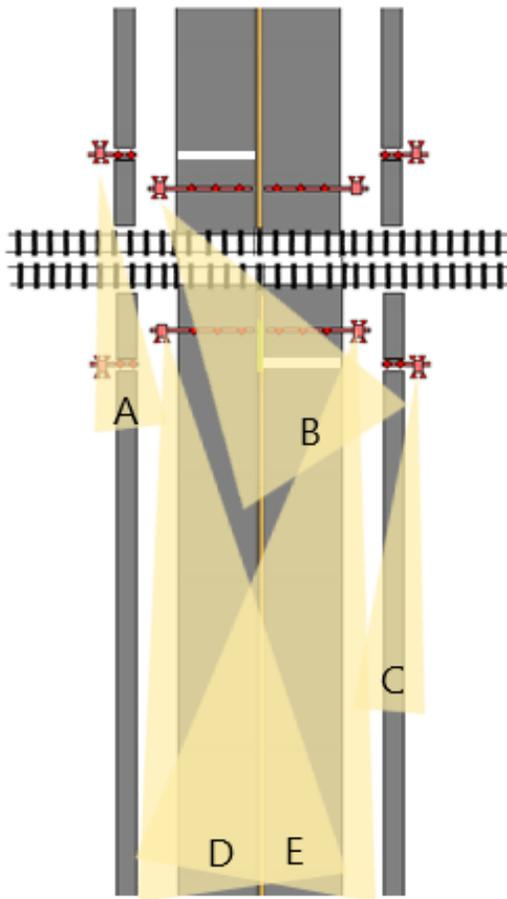
Alignment point at reference letter viewed at a height of 5 feet 6 inches above the road or sidewalk
