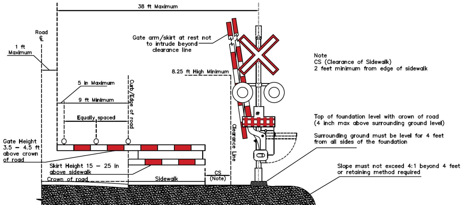
FIGURE 4-3: PEDESTRIAN & ENTRANCE GATE WITH SHARED MECHANISM
