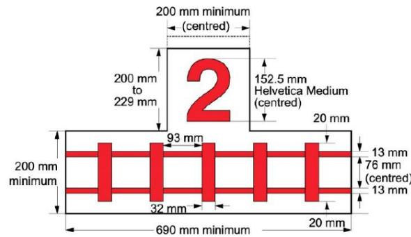
11.4.12 Number of Tracks signs shall be installed at both public and private Grade Crossings, with retro-reflective coating, symbols, and dimensions as specified in the GCH.
