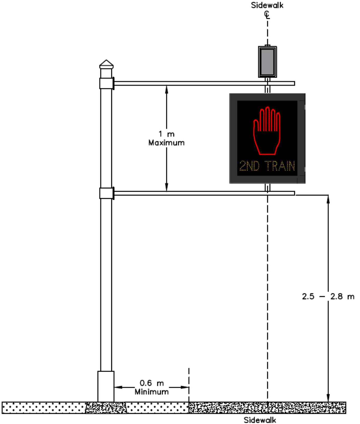
FIGURE 5-5: DYNAMIC MTWS CANTILEVERED OFF PEDESTRIAN GATE
