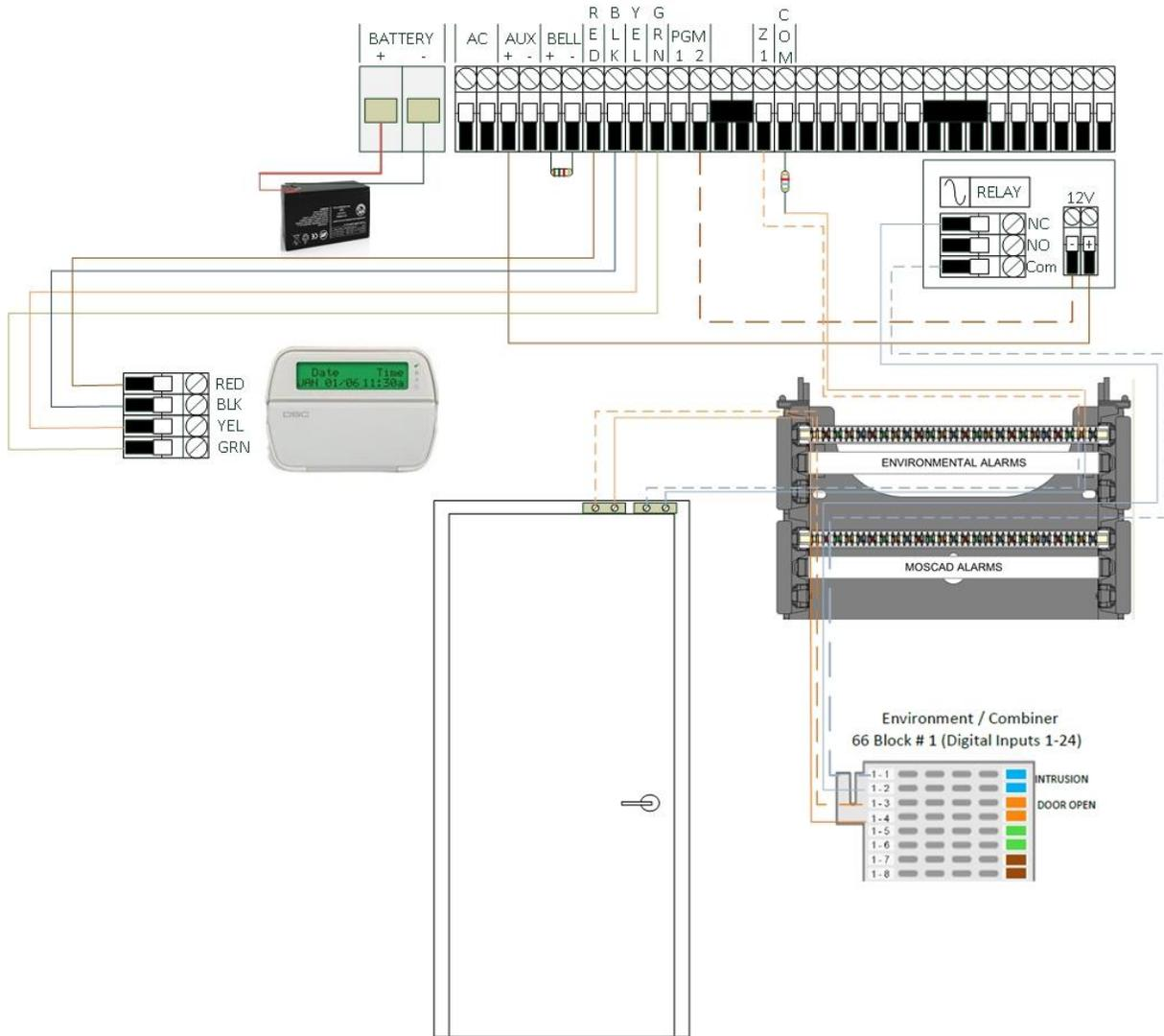
**Figure 16: Bix block cross connect**
