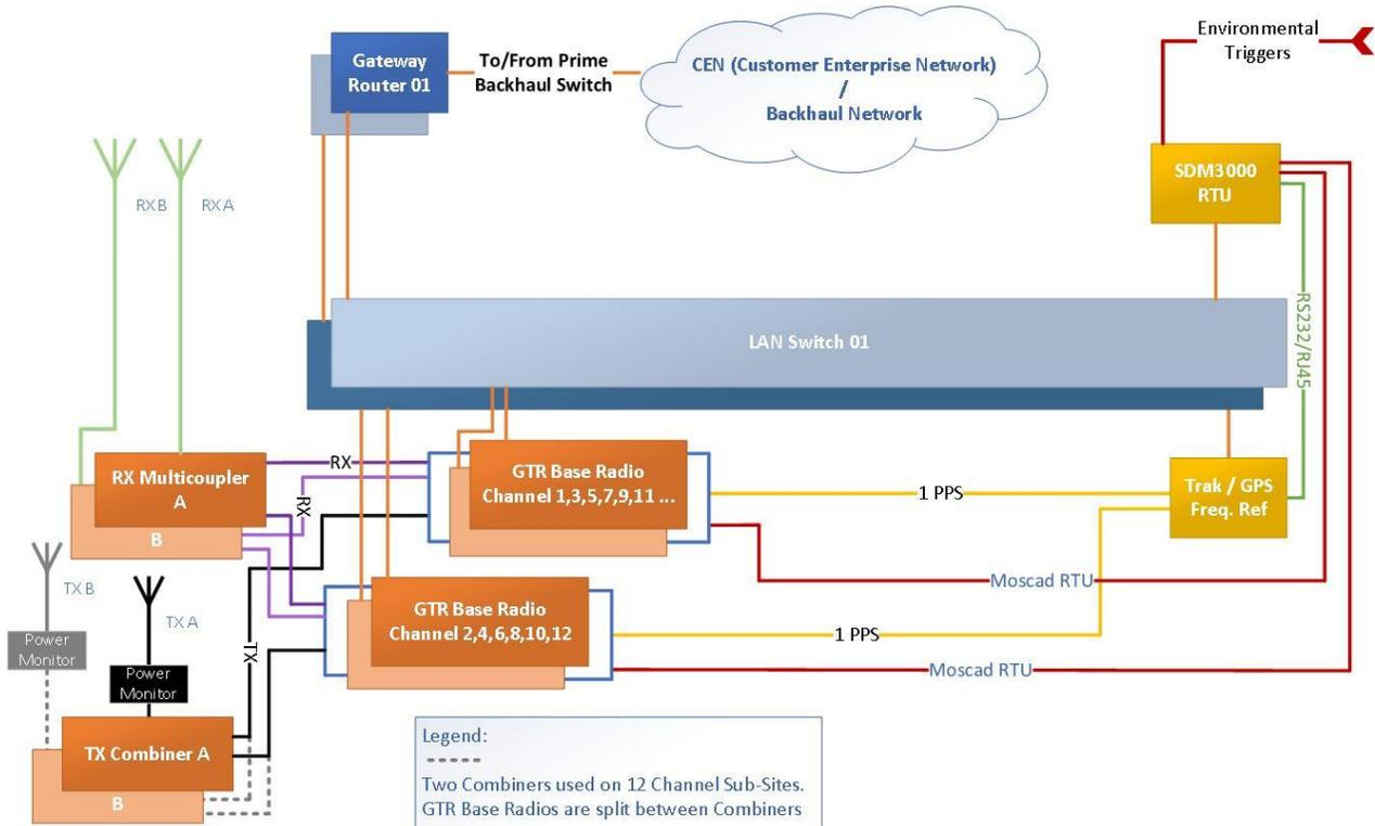
**Figure 4: Customer Enterprise Network (CEN)/ Backhaul Network - General Backhaul Network Setup**
