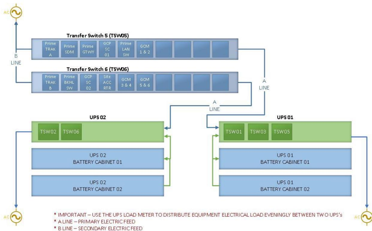
**Figure 22: Radio systems Prime Site 12-channel transfer switch and UPS diagram**
