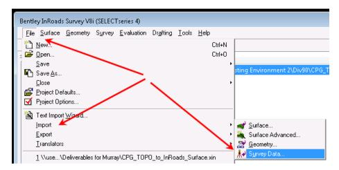
This will start a number of dialog boxes that will guide the user through the import process. This document will only focus on the what is needed to import the data. Other settings in the dialogs are left to the operator to define for the particular project.
