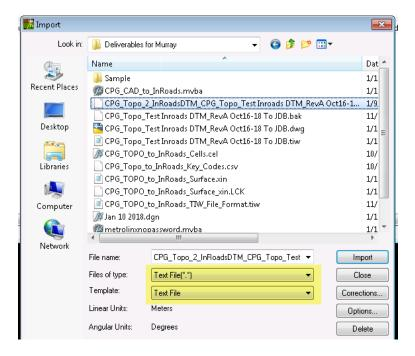
Ensure the file type is selected as "Text File" and the template as "Text File". Select the .out file that was created previously and press "Import".
