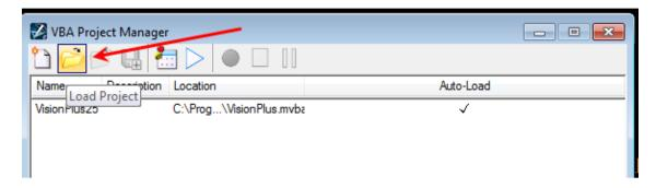
After pressing the Load Project Icon a file open dialog will open to allow the user to navigate to directory containing all the custom files for this process. The file extension filter will be for .mvba files. Select the file called "MX\_CADD\_toInRoads.mvba" and press open.
