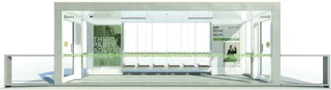
SHELTER TYPE 1 - RAIL LINE STATION PASSENGER SHELTER
