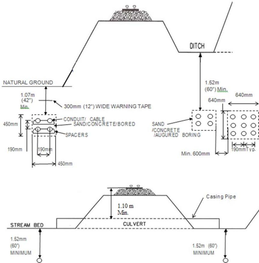
Figure 3: Cable Depth around Culverts and Ditches
