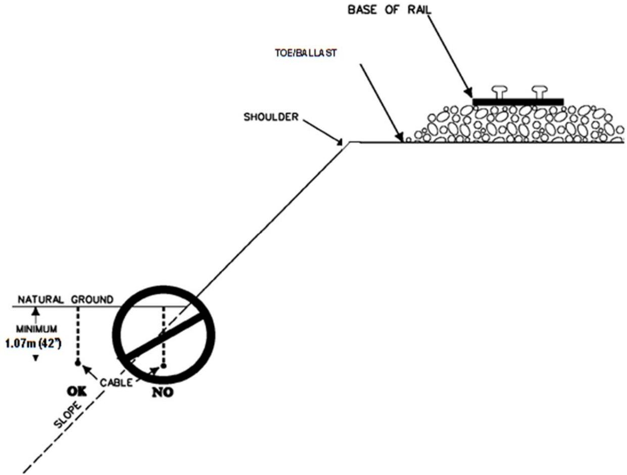
Figure 1: Fill Installation Directional Bore
