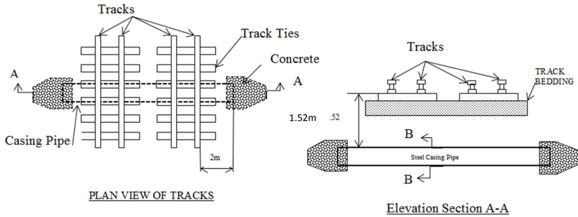
Figure 5: Cable Crossing Under Rail Tracks
