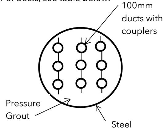
**Steel Casing Pipe (with 9 conduits)**
