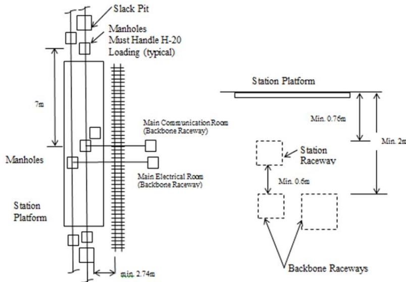
Figure 4: Cable Depth at Station Platform
