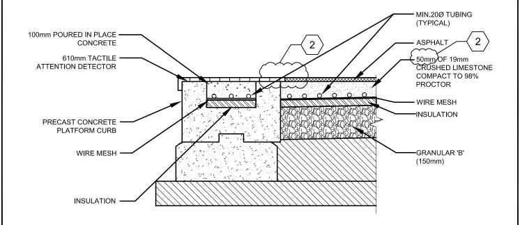
1 SNOW MELTING TUBING INSTALLATION DETAILS (ASPHALT PLATFORM)
