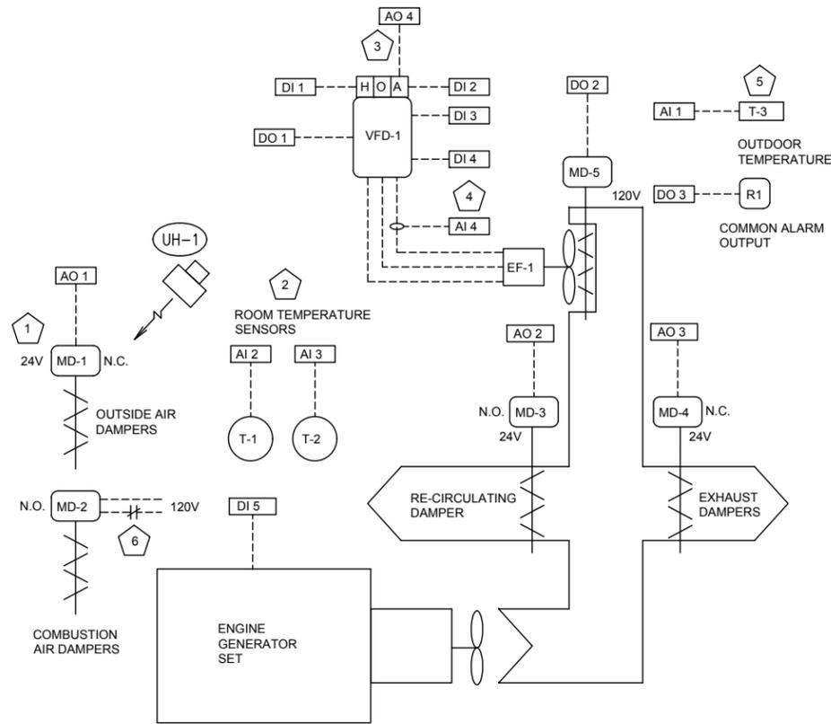
TEMPERATURE SENSORS T-1 AND T-2 ARE USED TO MAINTAIN THE TEMPERATURE IN THE GENERATOR ROOM. IF EITHER TEMPERATURE SENSOR FAILS, THE OTHER SENSOR WILL ASSUME CONTROL AND AN ALARM WILL BE GENERATED BY THE BUILDING AUTOMATION SYSTEM (BAS). OTHERWISE, THE AVERAGE OF THE TWO SENSORS WILL BE USED FOR CONTROL PURPOSES.
