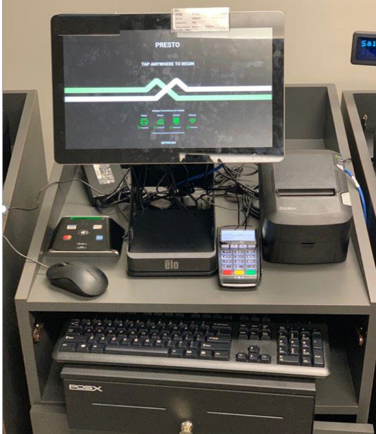
Figure 6: Fully Installed SPOS - Tabletop Stand
