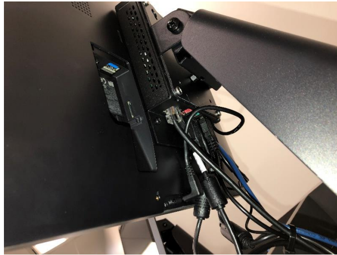
Figure 4: Mounting Option 1 - Mounting Arm with Expansion Module (Side View)
