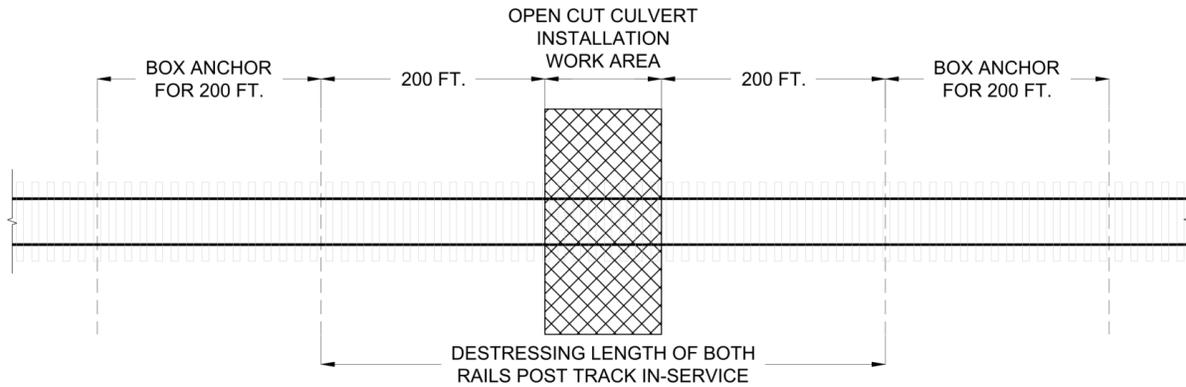
Figure 38-A. Destressing Length for Open Cut Culvert Installations
