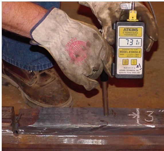
Figure 7-3: Measurement of Rail Temperature Courtesy CN Training
