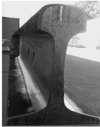
Figure 10-6: Machined Thick Web Rail to Match Standard Web
