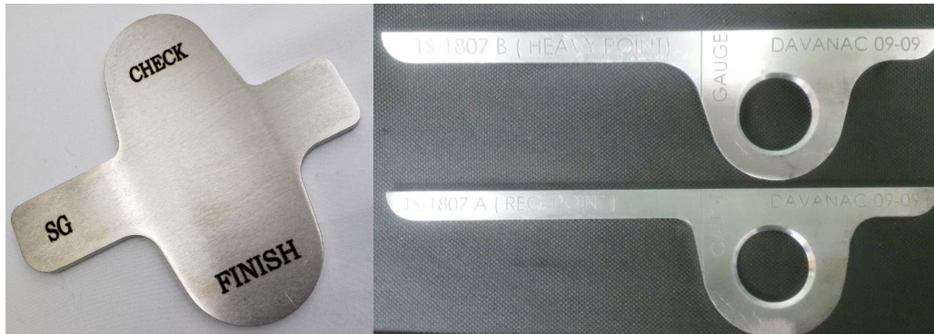
Figure 6-20: Flange and Radius Check Gauge, Heavy Point and Standard Point Flange Radius Gauge
