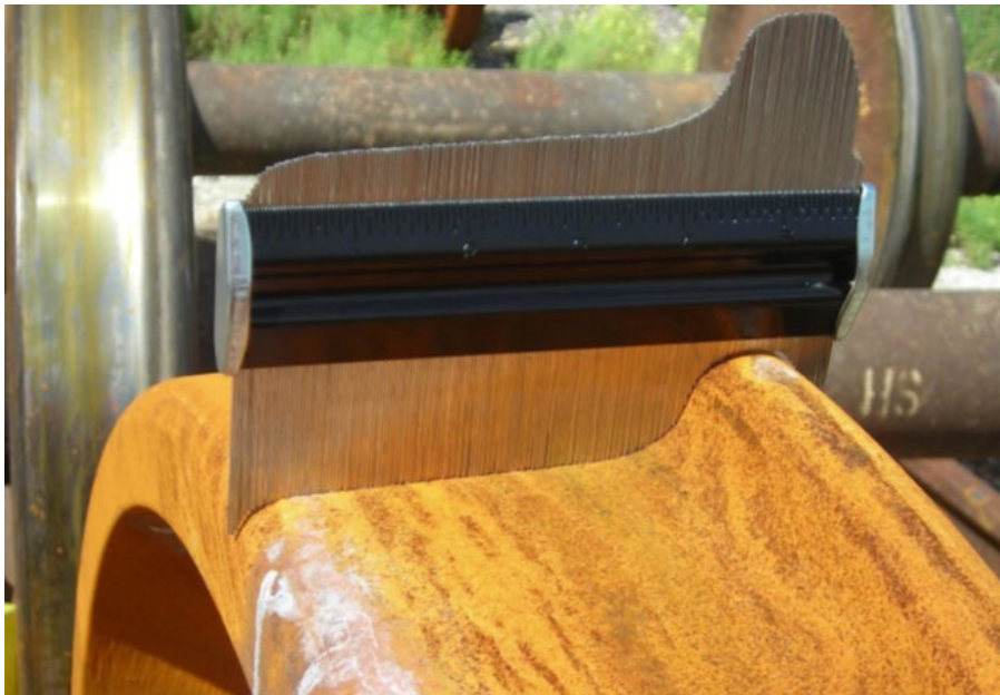
Figure 6-37: New Wheelset Gauge Showing Contour Wheel Tread Slope 1:20
