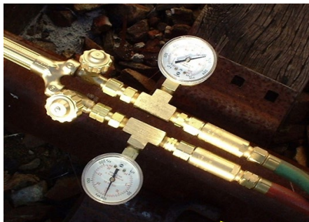
Figure 10-20: Position of In-line Gauges and Flashback Arrestors
