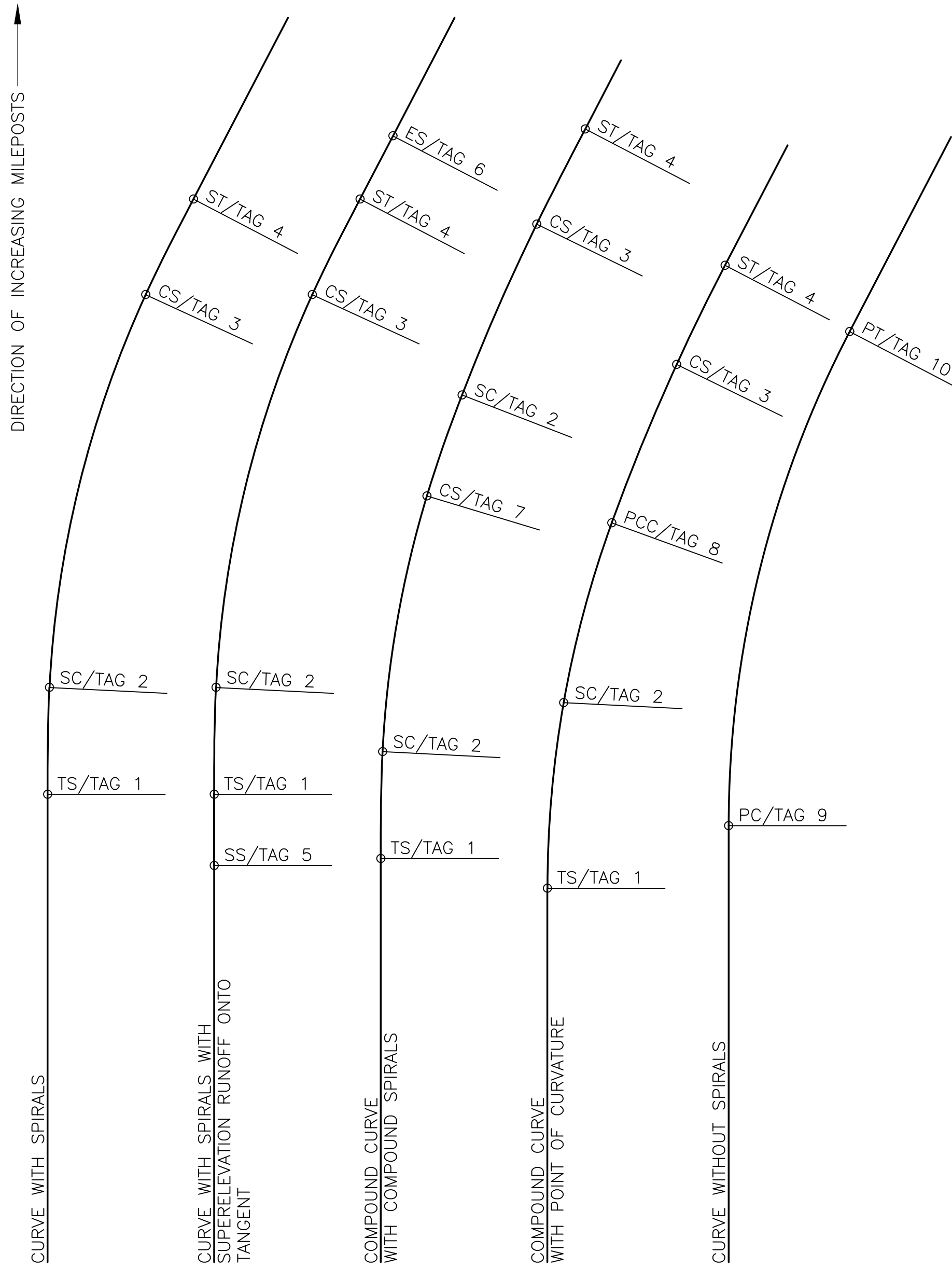
PLAN – LOCATIONS TO BE TAGGED NOTE: RH CURVE AS SHOWN, LH OPPOSITE
