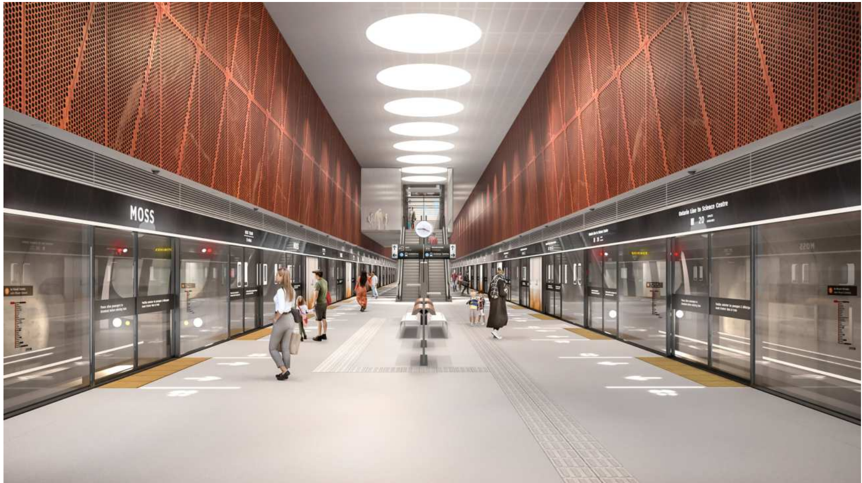
Figure 7-1: View from the below grade platform typology demonstrating the relationship between the feature walls, platform edge doors, digital signage, DWA area and overall look and feel of the platform. Renders are representational only.
