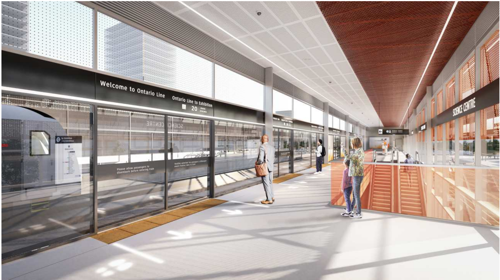
Figure 7-2: View from the elevated platform typology demonstrating the relationship between the feature ceilings, platform edge doors, digital signage and overall look and feel of the platform. Renders are representational only.
