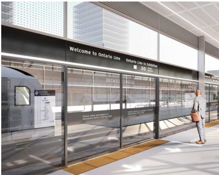
Figure 7-6: View from the elevated platform typology demonstrating the relationship between the platform edge doors, digital signage and lighting. Renders are representational only.
