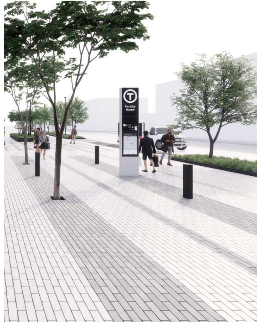
Figure 3-60: Bollards and Raised Planters as Traffic Barriers
