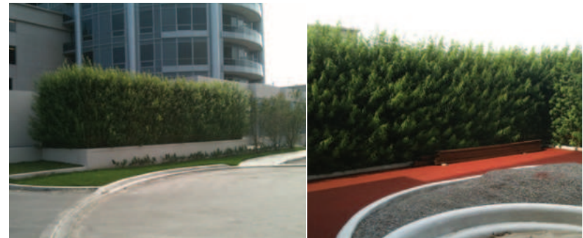
Figure 3-58: Living Wall Sound Barrier
