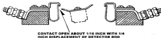
Figure 329(b)(2)- 4: GRS Switch Machine Point Detector Contacts.
