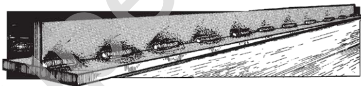
Figure 8.15-Staggered intermittent welds/ chain intermittent welds
